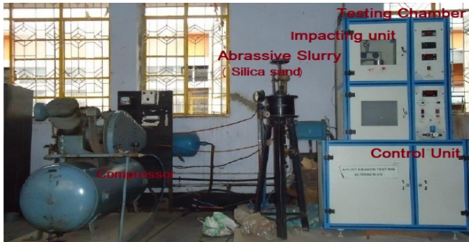
Fig. 2. Set up for Erosion Test
