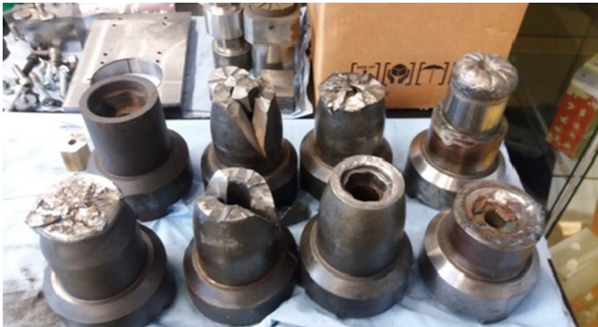
Fig. 1. Damage of dies and handles during the KOBO extrusion
