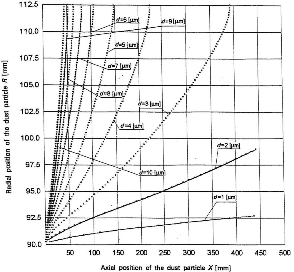
Fig. 4. Trajectories of the spherical dust particles for the axial speed varying in radial direction
