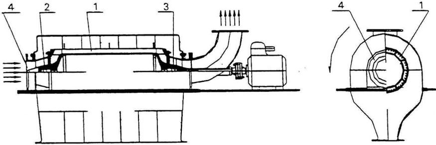
Fig. 9. Radial cross-section of the dust separator
