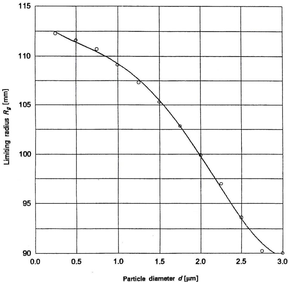
Fig. 7. Limiting radiuses  $R_g$  as a function of the dust particle sizes  $d$
