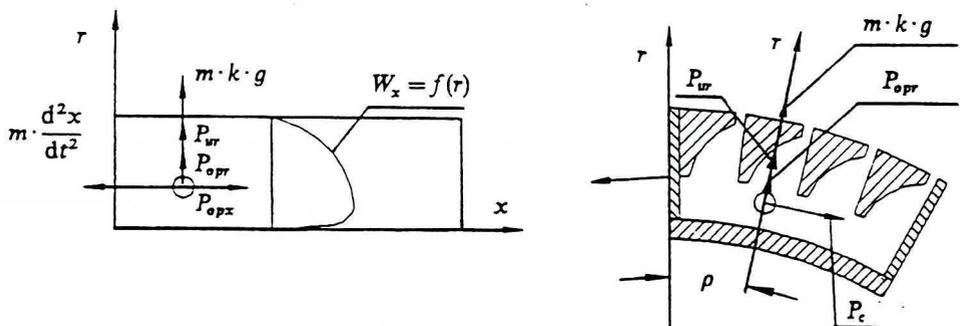
Fig. 2. Details of the forces acting on a dust particle within rotating channel of the rotor
