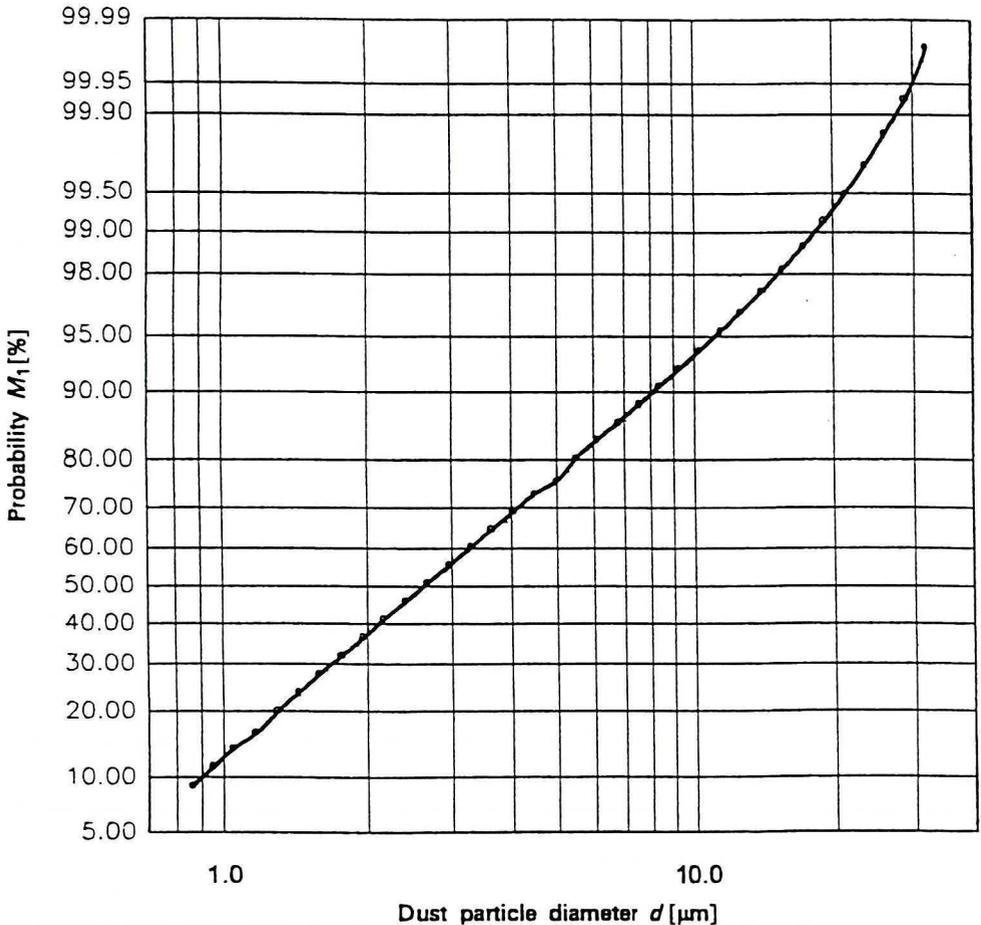
Fig. 5. Probability density of the dust particle sizes
