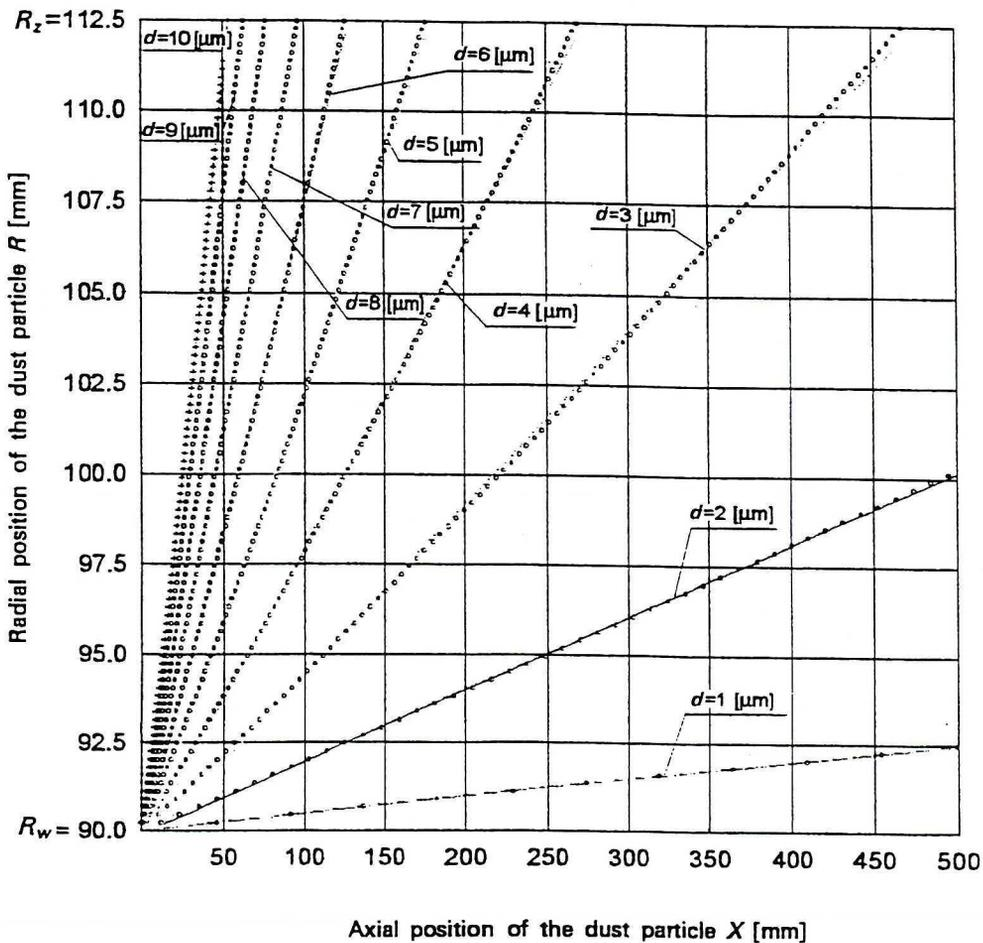
Fig. 3. Trajectories of the spherical dust particles for a constant axial speed
