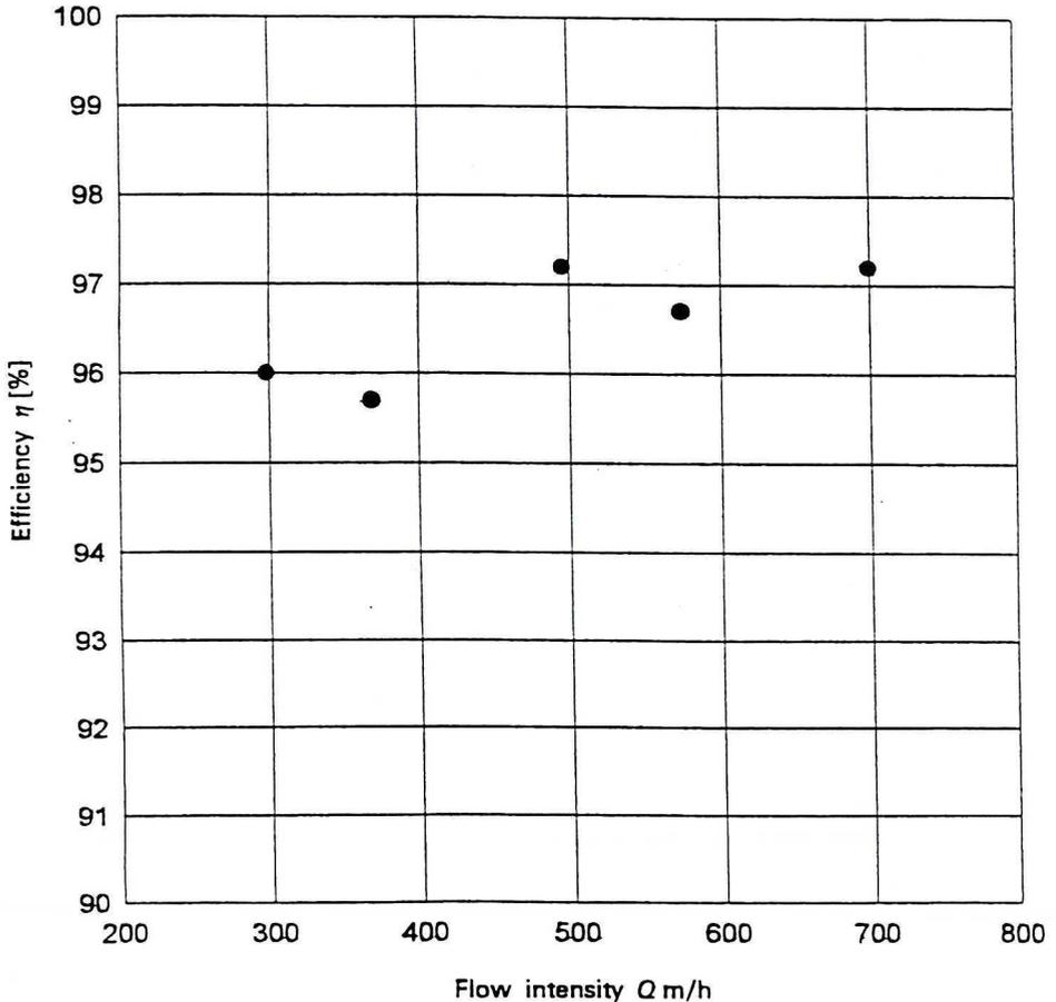
Fig. 11. Flow rate variations versus the dust separation efficiency
