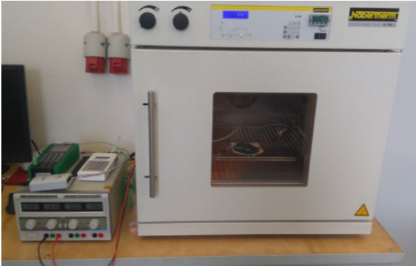
Fig. 10. Test of RTD installed on PCB
