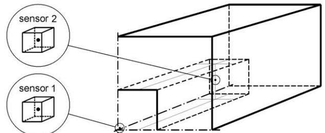
Fig. 2. Domain considered – casting of cuboid shape
