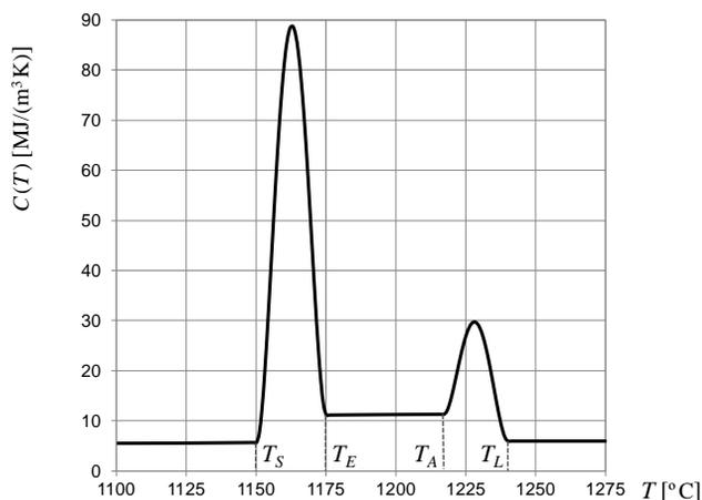
Fig. 3. Substitute thermal capacity of cast iron
