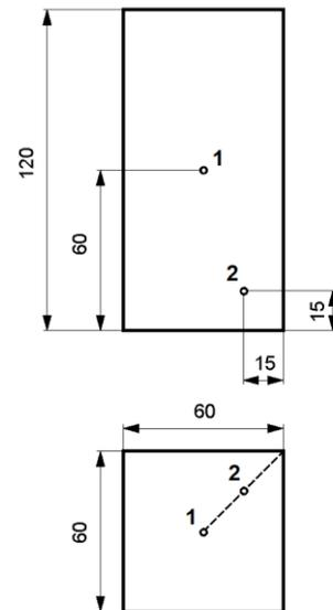
Fig. 1. Test casting – cuboid
