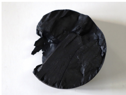
Fig. 5. Dull brown coal, borehole WSx, sample 3 – depth 468 m
