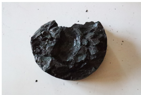
Fig. 4. Bright brown coal, borehole WSx, sample 2 – depth 470 m
