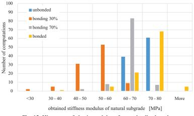
Fig. 12. Histogram of elastic modulus of natural soil subgrade
