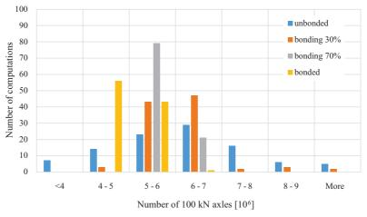
Fig. 16. Histogram of durability due to asphalt fatigue cracks
