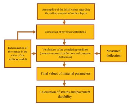
Fig. 1. Scheme of backcalculation process
