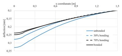
Fig. 6. Pavement deflections with various bonding condition
