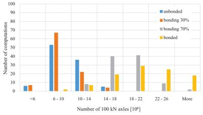
Fig. 17. Histogram of durability due to structural ruts
