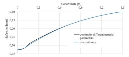
Fig. 9. Deflections of the road surface with and without bonding for different material parameters
