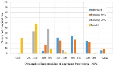
Fig. 11. Histogram of modulus of elasticity of aggregate base course
