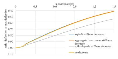
Fig. 8. Influence of the weakening of individual pavement layers on the shape of the deflection basin
