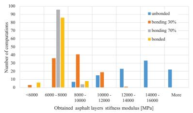
Fig. 10. Histogram of obtained elasticity modulus of asphalt layers
