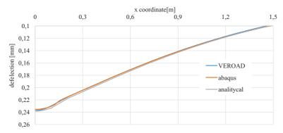
Fig. 4. Pavement deflections for models with bonded layers from FE calculations, VEROAD calculations and implementation of the Hankel transform solution
