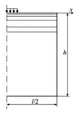
Fig. 2. Section of a axisymmetric cylindrical domain of a pavement modelled using FEM
