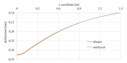
Fig. 5. Pavement deflections in the absence of adhesion between the binder course and the asphalt base course using, FEM and Hankel transform
