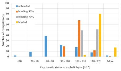
Fig. 14. Histogram of maximum tensile strains of the asphalt layer
