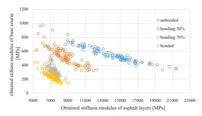
Fig. 13. Obtained values of moduli of asphalt layers and aggregate base course
