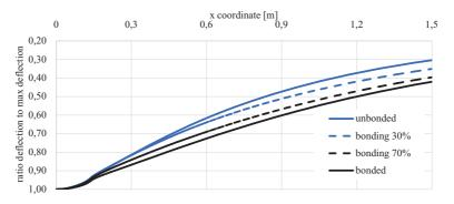
Fig. 7. Ratio of pavement deflections to maximum deflection with various bonding condition
