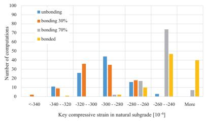
Fig. 15. Histogram of maximum compressive strains in the natural subgrade
