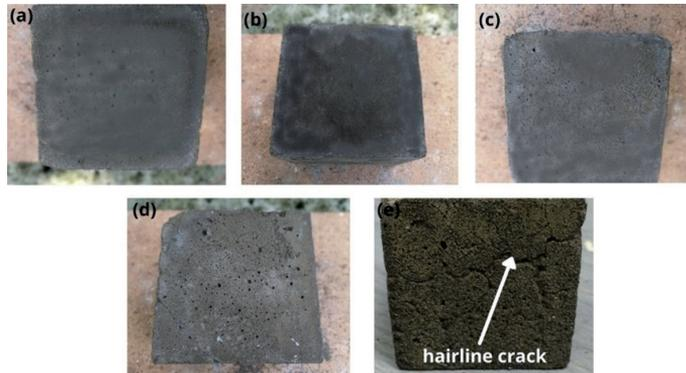
Fig. 3. Visual surface appearance of (a) CRGM-0, (b) CRGM-5, (c) CRGM-10, (d) CRGM-15 and (e) CRGM-20 after temperature exposure at 400°C
