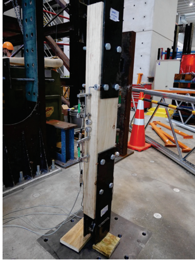
Fig. 11. Specimen configuration in bolted connection test done by [12]
