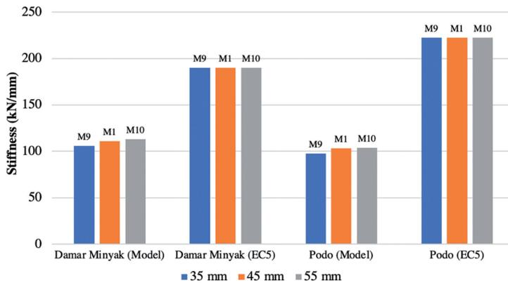
Fig. 19. Stiffness versus edge distance
