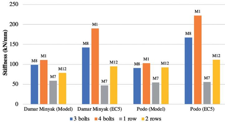
Fig. 18. Stiffness versus number of bolts and rows
