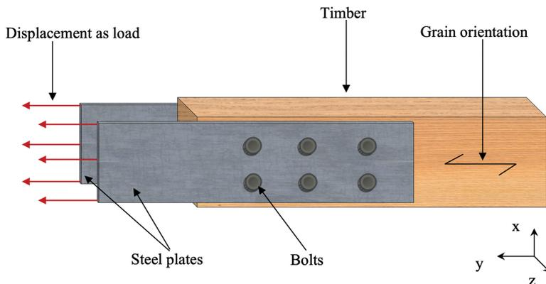
Fig. 1. Steel-wood-steel connection loaded parallel to grain [12]
