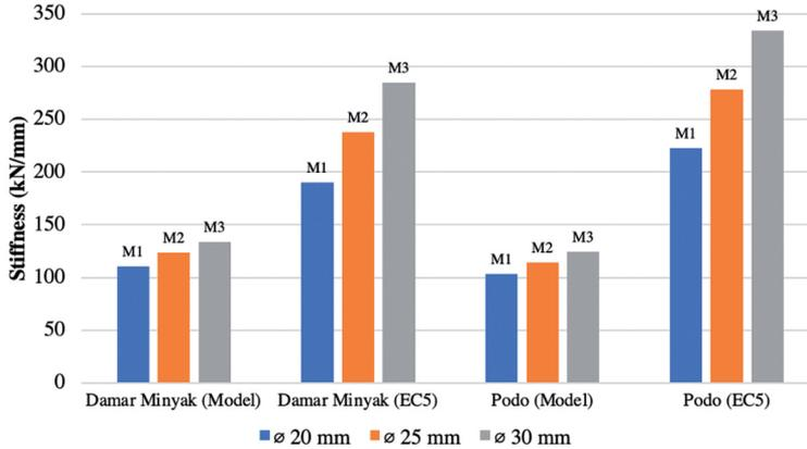
Fig. 15. Stiffness versus bolt diameter
