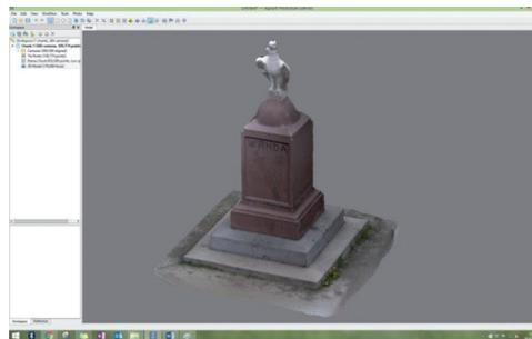
Fig. 3. The finished model after reconstruction and texturing in Agisoft PhotoScan
