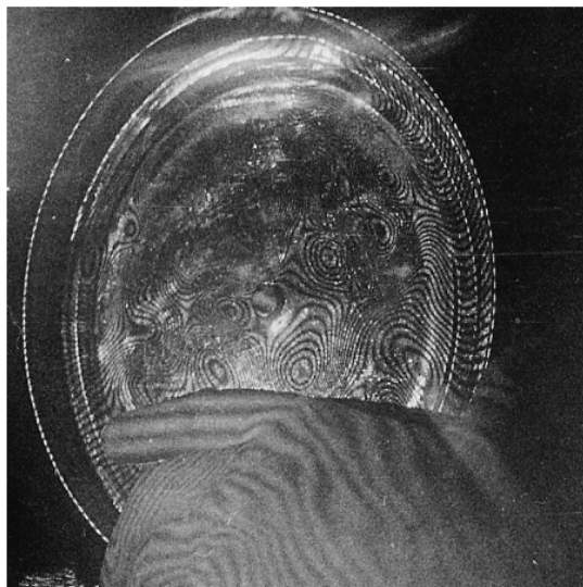
Fig. 19. A reconstructed interferogram of a hand-held membrane, created using a holocamera system with a double-pulsed ruby laser. For medical applications, the distributions of the band field are of interest – in the photograph, these are the bands on the hand holding the membrane [24].
