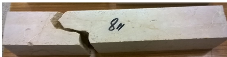
Fig. 7. A sample with dimensions of 50×50×300 mm after the flexural strength test with visible cracks within the so-called stylolite seams
