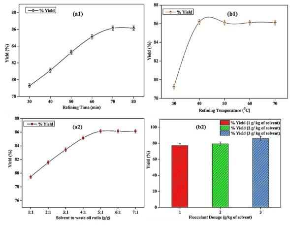
Fig. 3. Effect of (a1) refining time (b1) refining temperature on percentage yield of recovered oil (a2) solvent to waste oil ratio (b2) flocculant dosage on yield% of recovered oil
