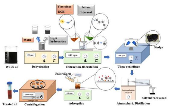
Fig. 1. Process flow diagram of extraction-flocculation process
