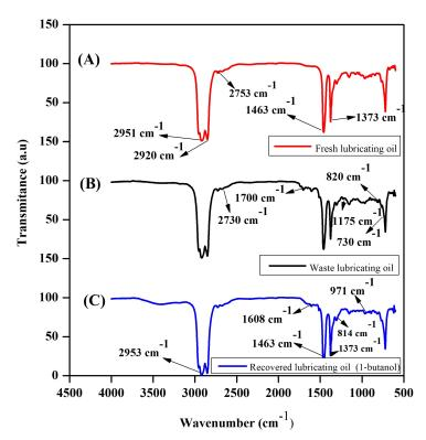
Fig. 4. FTIR analysis of fresh, used and recovered lubricating oil
