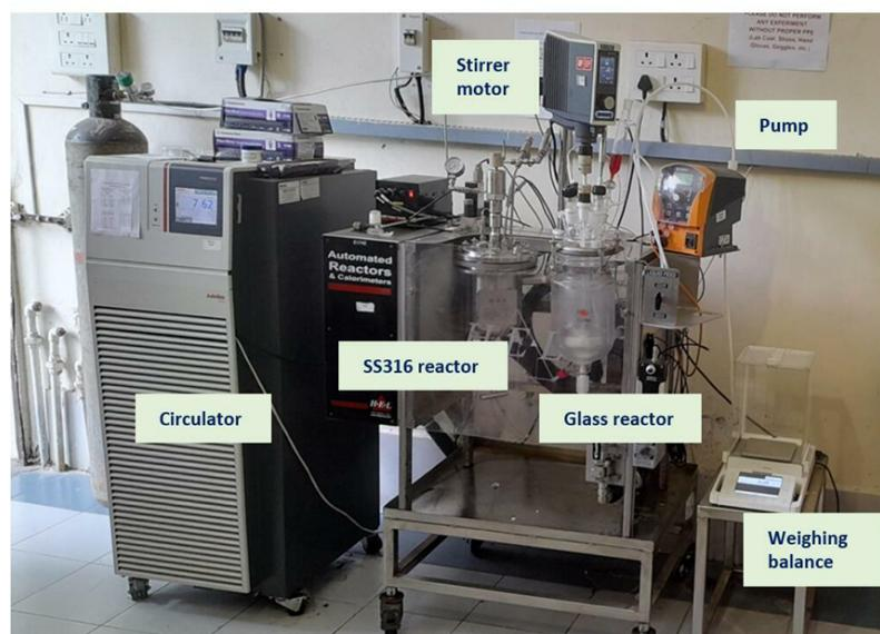
Fig. 1. Reaction calorimeter used for the experiments
