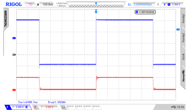
Fig. 8. VTP1220FBH current response for a 1000 Hz square PWM signal.
