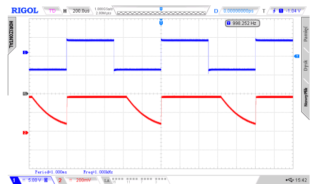
Fig. 3. Grove Light Sensor v1.2 voltage output signal for a 1000 Hz square PWM signal.
