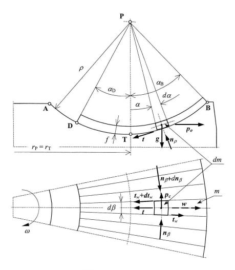
Fig. 9. Forces of the layer element in a motion without a slip
