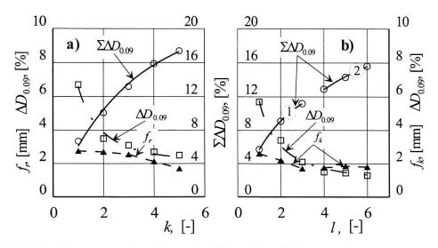
Fig. 6. The influence repeated crushing on the effect and layer thickness. a) roller  $-d_r = 150$  mm, s = 231 kPa,  $f_0 = 8$  mm, b) ring-ball assembly  $-d_k = 100$  mm,  $s_k = 115$  kPa,  $\omega = 8.2$  1/sec
