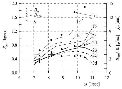
Fig. 11. Flow and efficiency of a grinding assembly without ventilation for:  $z_k = 7$ ,  $\alpha_A = \alpha_B = 45^\circ$ ,  $s_k \approx 68$  kPa,  $\mu = 0.40$ ,  $\mu_w = 0.65$ ; a – the effect of the stream in the direction  $\alpha - n_{\alpha,D}$  and f = constant; b – according to the modelling conditions and f = constant; c – exemplary linear distribution of the layer; d – experimental results
