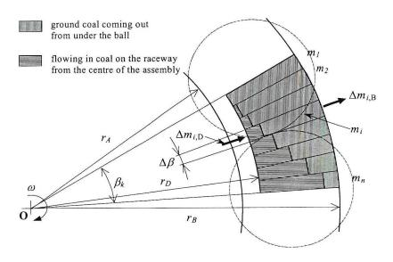
Fig. 10. Flow visualization of coal on the active arc of the raceway
