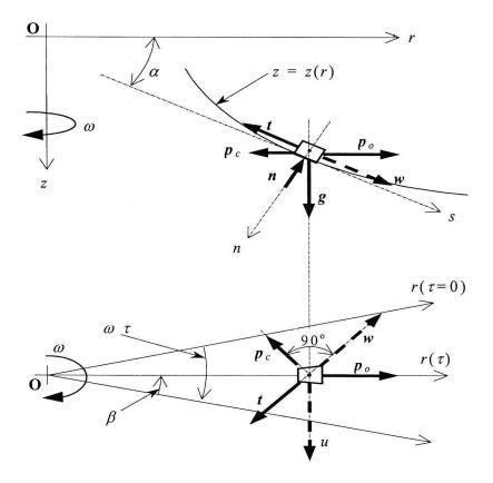
Fig. 8. Diagram of forces and velocities in a relative axi-symmetric motion
