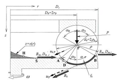
Fig. 7. Characteristics of the grinding assembly
