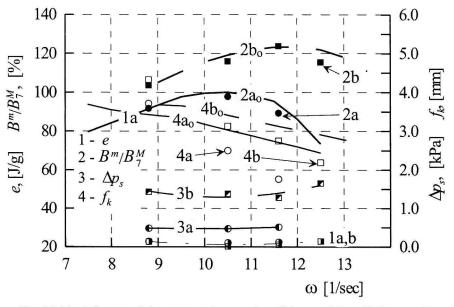
Fig. 15. The influence of the raceway slope on the efficiency of the mill for:  $z_k = 7$ ,  $s_{k,1} = s_{k,2} = 157$  kPa,  $a - \alpha_A = \alpha_B = 45^\circ$ ,  $b - \alpha_A = 30^\circ$ ,  $\alpha_B = 60^\circ$ . Subscript " $_{o}$ " – calculations
