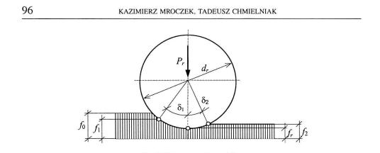
Fig. 2. Geometry of crushing
