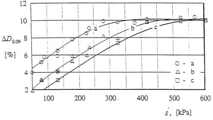
Fig. 5. The influence of pressure on the grinding effect of the size class  $0\div 2 \text{ mm}$  by  $f/d_r = 4\%$ . a – primary crushing, b – secondary crushing after screening of the size class  $0\div 0.2 \text{ mm}$  (dust), c – third crushing after repeated screening of dust
