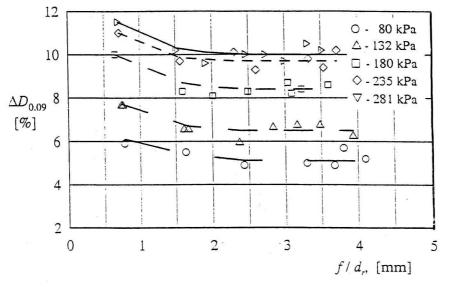
Fig. 4. The effect  $\Delta D_{0.009}$  – layer thickness relations at different unit-pressures under the roller  $d_r = 150$  mm, primary crushing
