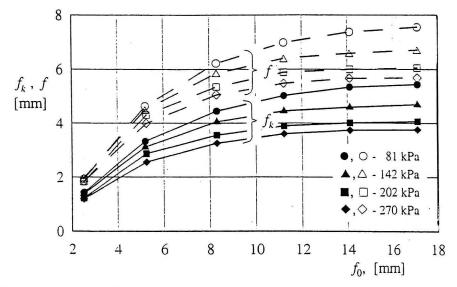
Fig. 3. The thickness of the drawn-in layer as a function of its initial thickness ( $d_r = 125$  mm), (Pulling conditions of the coal layer)
