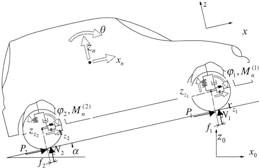
Fig. 4 Model of a car
