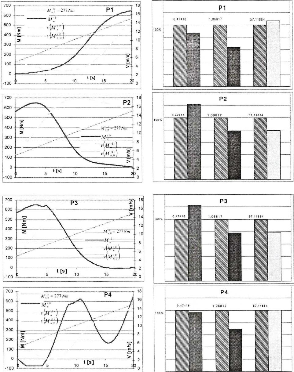
Fig. 8 Courses of drive moment and velocity of the car for task 1, cases P1, P2, P3, P4.
