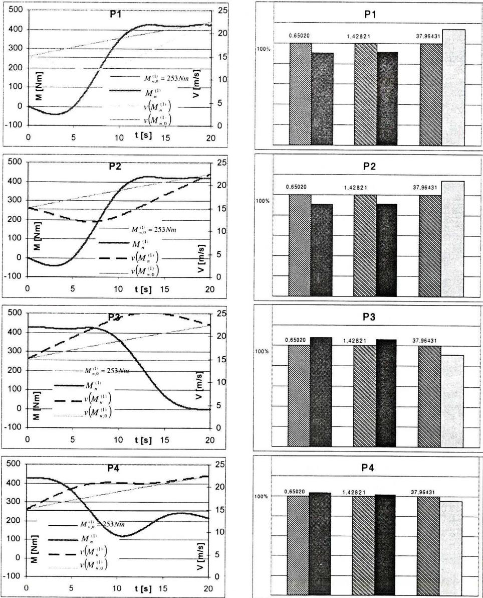
Fig. 11. Courses of drive moment and velocity of the car for task 2, cases P1, P2, P3, P4. LPG feed
