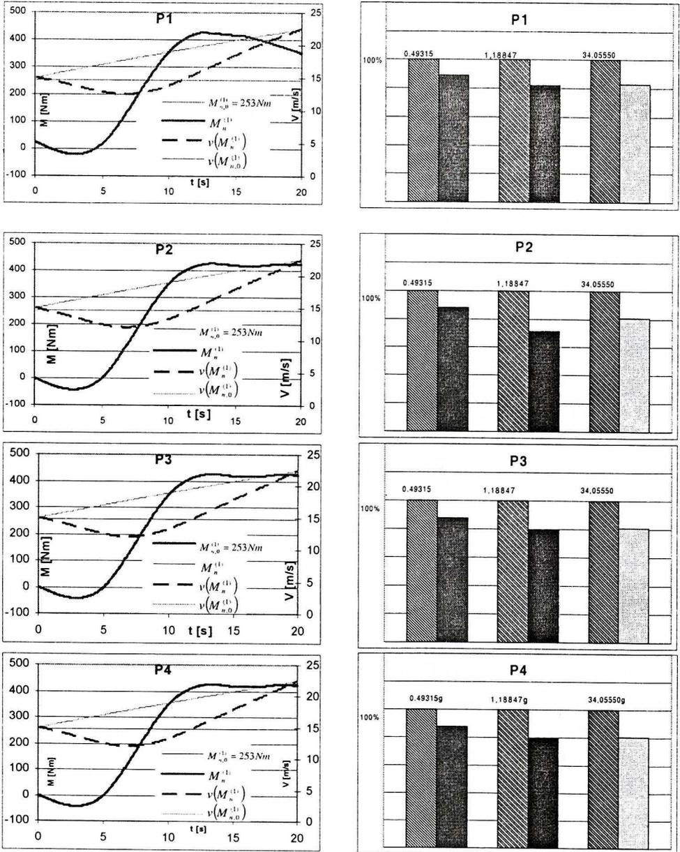
Fig. 10 Courses of drive moment and velocity of the car for task 2, cases P1, P2, P3, P4. Petrol feed
