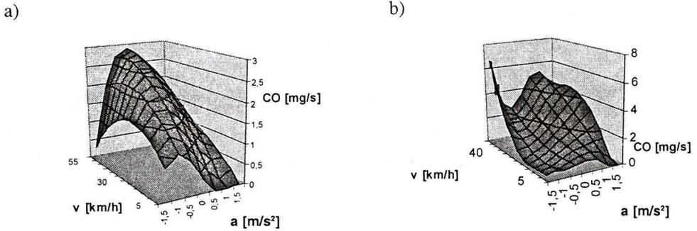
Fig. 2. Averaging dynamic characteristics of carbon monoxide emission: a) petrol, b) LPG
