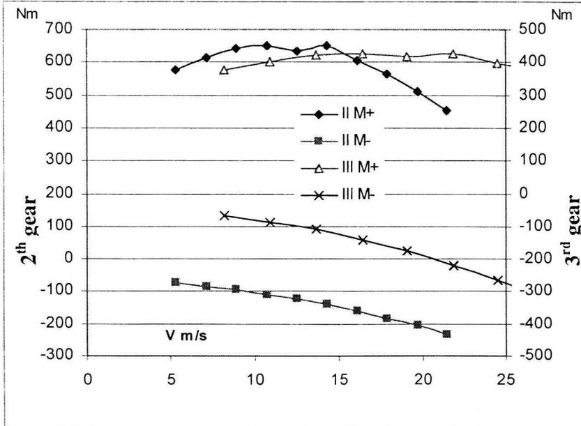
Fig. 6. Limitations of the drive moments for the second (II) and third (III) gear
