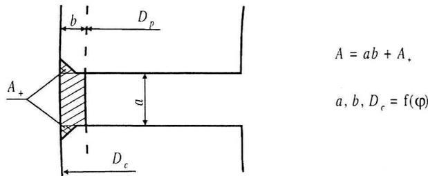
Fig. 4. A scheme to calculate the area of a ring-end gap ( $\varphi$  – crankshaft angle)
