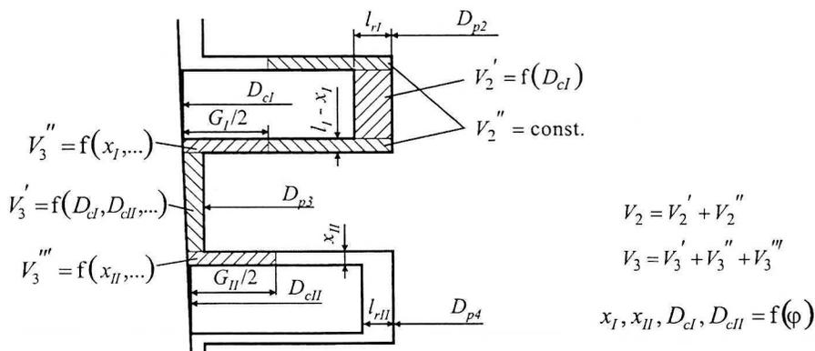
Fig. 7. A scheme to calculate the volumes of regions (for example the regions: behind the top ring and between the top and the second ring)
