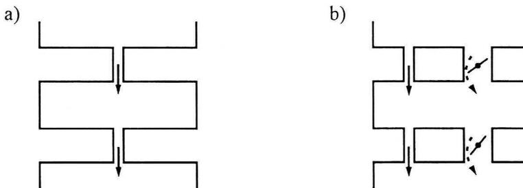
Fig. 1. Schematic diagram of labyrinth seal, considering gas flow only through the ring gaps (a) and gas flow through the ring gaps and through the grooves around the rings – the areas of the gas flow through the grooves are determined by axial position of the rings in the groove, but cumulative action of volumes behind the rings is not considered (b)
