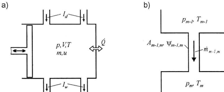
Fig. 3. Schematics of a single labyrinth stage (a) and an orifice linking two regions (b) ( $I_d$  and  $I_w$  – enthalpy of the gas incoming and outgoing in the region, respectively,  $\dot{Q}$  – heat transfer rate over the boundary of a control volume,  $\psi$  – flow coefficient)
