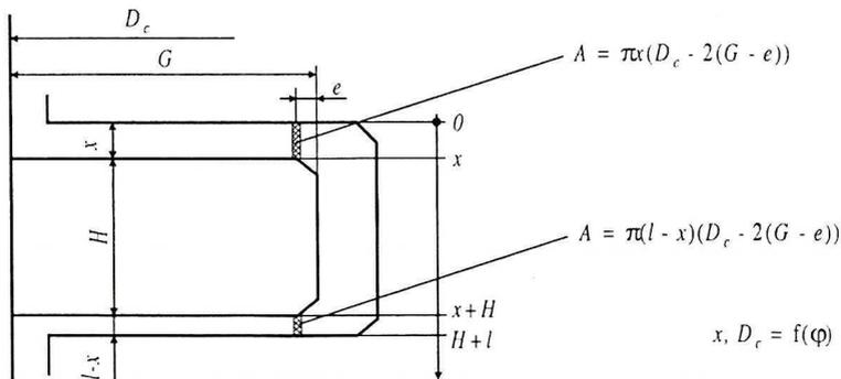
Fig. 5. A scheme to calculate the cross-section area of side-ring crevices
