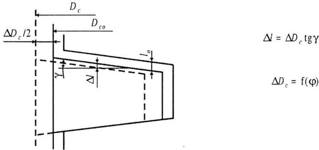
Fig. 6. Effect of the cylinder diameter on the axial clearance of a keystone ring
