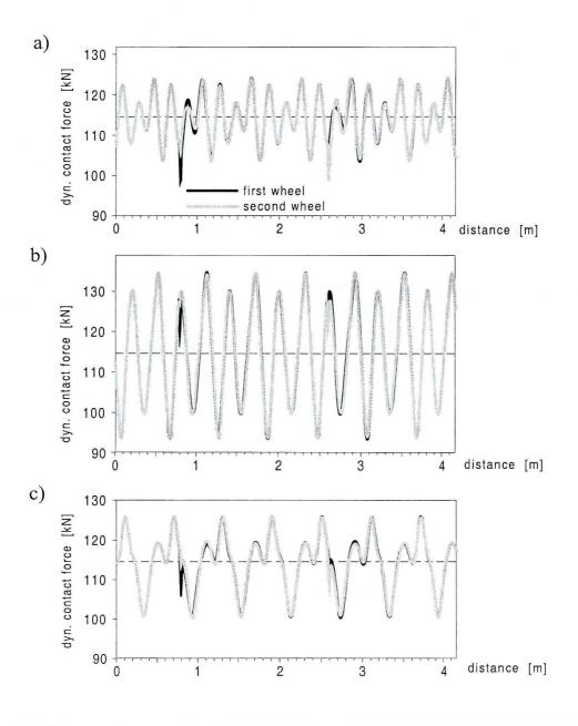
Fig. 7. Wheel-rail dynamic contact forces due to the passage along the "squat"-type crack in the rail for travelling speeds: (a) 60, (b) 80 and (c) 120 km/h
