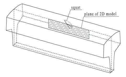
Fig. 1. The "squat"-type crack in the rail tread and its representation in the rail 2D-model
