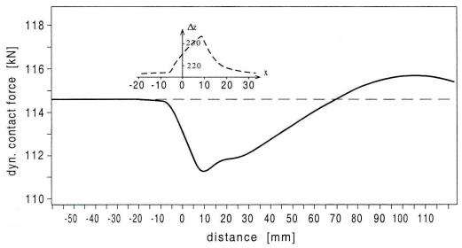
Fig. 10. Dynamic contact force for the first bogie wheelset wheel rolling with the travelling speed 60 km/h along the even rail with the kinematic excitation caused by the crack in the tread demonstrated together with the plot of cylinder vertical displacement expressed as the function of wheel position
