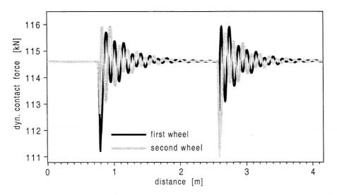
Fig. 8. Transient component of the bogie track dynamic response caused by the rail unevenness of the "squat"-type
