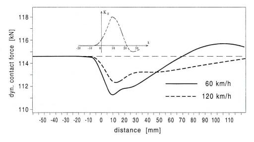
Fig. 9. Dynamic wheel-rail contact force for the first bogie wheelset wheel rolling along the even rail with the kinematic excitation representing a crack in the tread. Stress intensity factor  $K_{II}$  for the quasi-static rolling of the cylinder along the cracked prism in the domain of cylinder position
