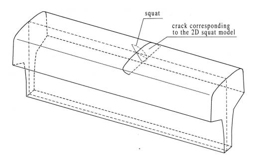
Fig. 2. Interpretation of the half-elliptical "squat"-type crack for analysis using the 2D model
