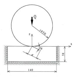
Fig. 3. Scheme of the 2-D cracked rail model with the railway wheel
