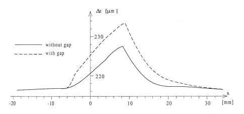
Fig. 5. The vertical displacement of the center of cylinder in domain of the cylinder current position
