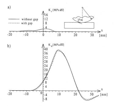
Fig. 4. Histories of the stress intensity factors during quasi-static rolling of the cylinder along the cracked prism
