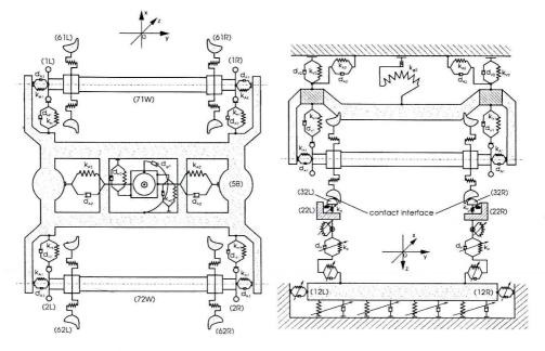
Fig. 6. Discrete-continuous model of the railway bogie-track system
