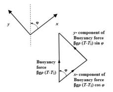
Fig. 1. Definition of the components of Buoyancy force
