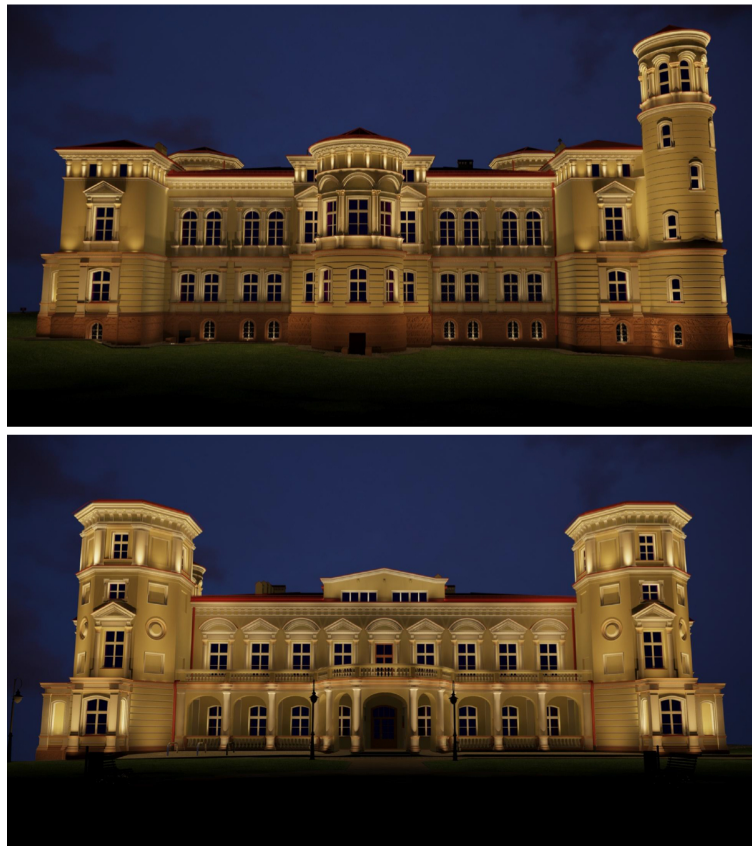
Fig. 10. Visualization of the illumination of both facades of the Lubomirski Palace using small luminaires
