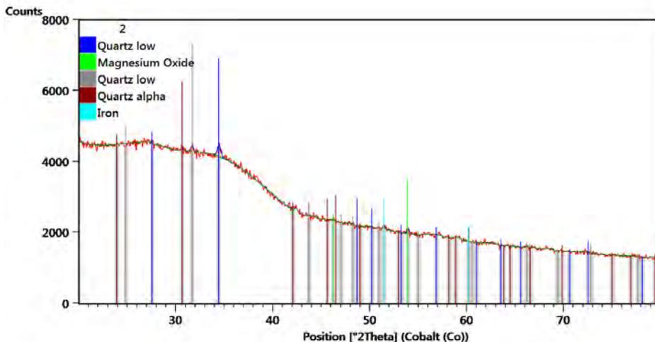
Fig. 7. X-ray diffraction pattern of blast furnace slag
