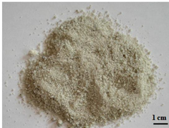
Fig. 1. Granulated blast furnace slag
