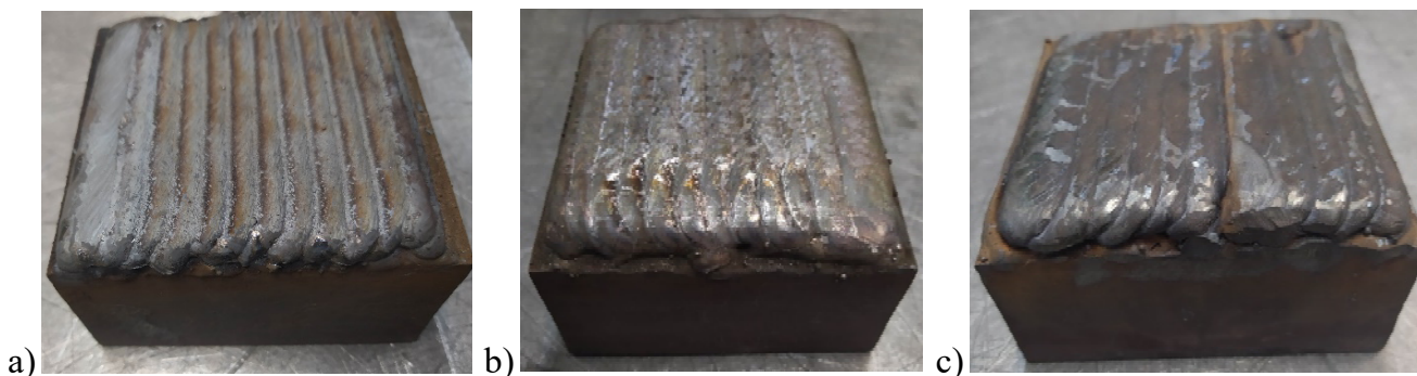
Fig. 14. Photographs of samples after the surfacing process: a) DO*341, b) DO*04, c) DO*15
