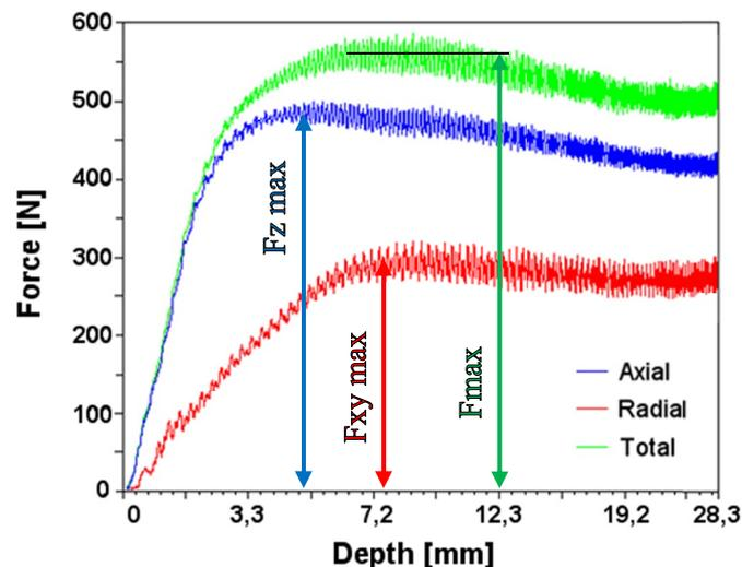
Fig. 5. Component force plot with reference to time
