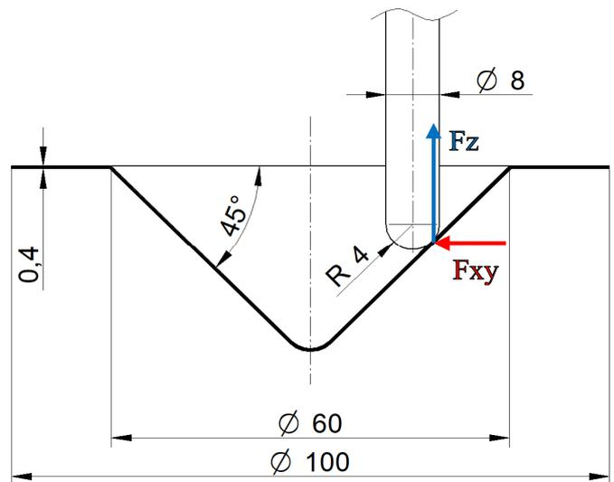
Fig. 2. Specimen geometry and forming force distribution
