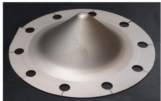
Fig. 3. One of the successfully obtained drawpieces
