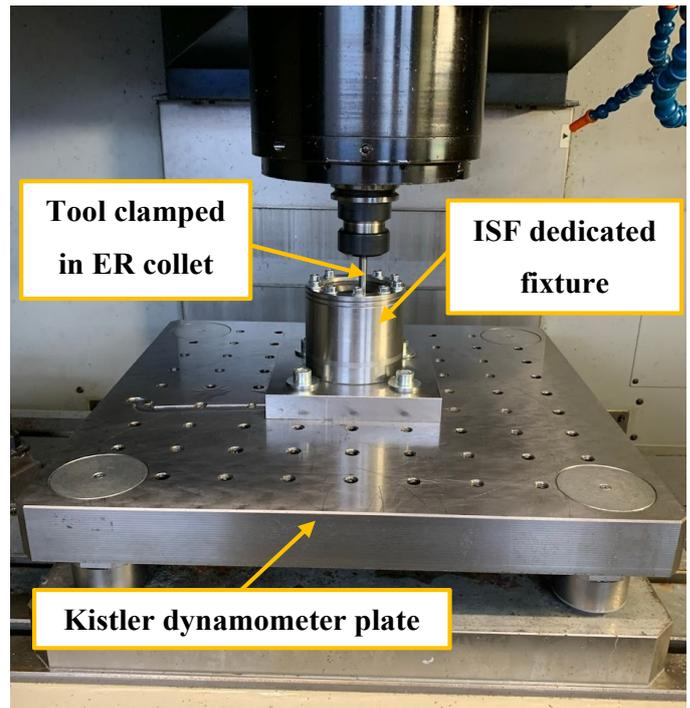
Fig. 1. Test stand for the ISF process
