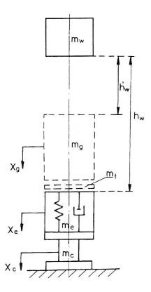
Fig. 2 Schematic diagram of the force transducer calibration system
