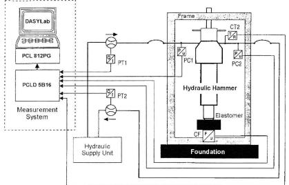
Fig. 3 Schematic diagram of the stand for measurement of hammer external parameters
