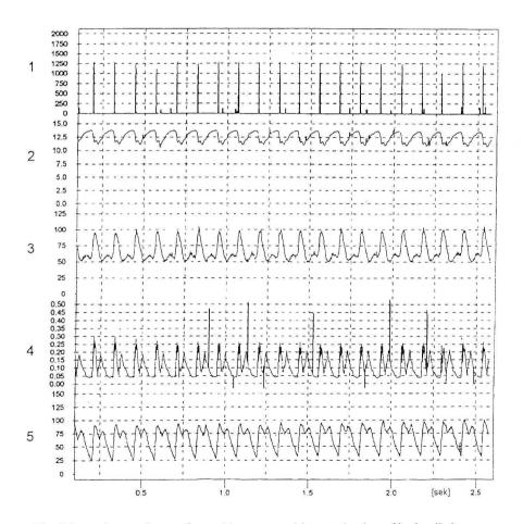
Fig. 5 Example waveforms of quantities measured in examination of hydraulic hammer *I* – energy; Nm, 2 – supply pressure, MPa; 3 – supply flow, dm<sup>3</sup>/min; *4* – run-off pressure, MPa; 5 – run-off flow, dm<sup>3</sup>/min
