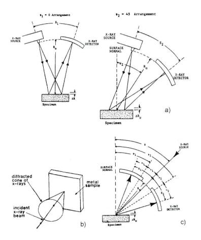
Fig 10 Schematic diagrams of X-ray technique arrangements a) double-exposure arrangement;
