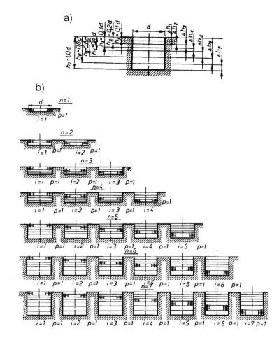
Fig. 5 Determining the computational coefficients for the hole-drilling method (according to Refs [9] and [10]); a) the assumed increments of the drilled hole, b) the problems solved to obtain coefficients  $A_{in}$  and  $B_{in}$  for each step of the hole deepening
