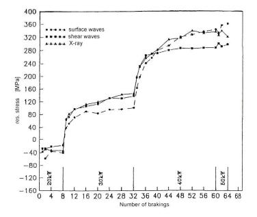
Fig. 14 The change in the circumferential residual stress component in the train wheel head due to multiple brakings of different power
