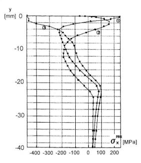
Fig. 15 The 2-D residual stress distribution due to the friction elastic-plastic rolling process of the steel strip, obtained by the FEM computation (according to Ref. [41]): ① - free rolling,
