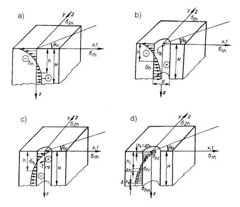
Fig. 4 The principle of the hole-drilling method (according to Ref. [9]); a) residual stress existing in the material, b) the reactions which should be applied at the surface of the drilled hole,c) applying the stresses with opposite sign, d) approximation of the real stress distribution
