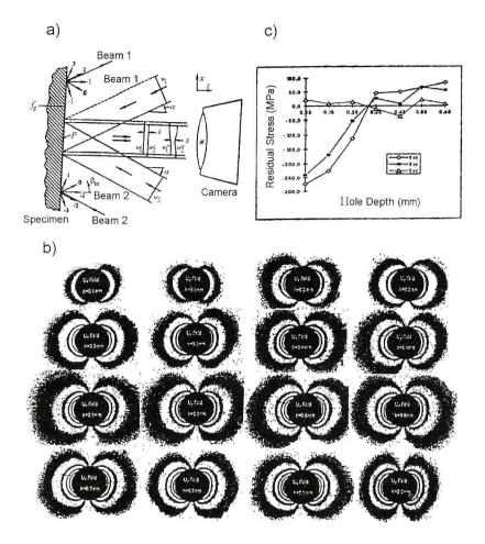
Fig. 6 The hole drilling method: surface displacement measurements provided by moiré interferometry (according to Ref. [15]); a) the principle of the measurement,b) displacements contour maps, c) the residual stress distribution inside the material
