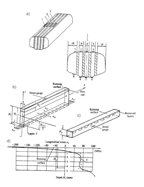
Fig. 3 The sectioning / layer removing method for determining residual stress in a rail head (according to ref. [4]): a) cutting the rail head into plates; positions of strain gages,
