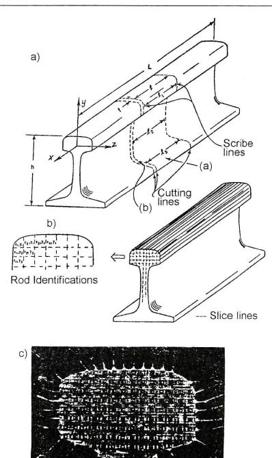
Fig. 1 The sectioning method for determining residual stress in rails (according to Ref. [2]),a) two specimen cut out from a rail portion, b) sectioning of the specimen (a) into long bars, c) rosettes of strain gages at the face of the thin slice
