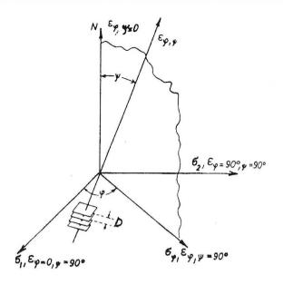
Fig. 9 Symbols used in X-ray strain measurement
