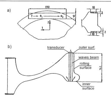
Fig. 13 Ultrasonic techniques for residual stress measurements in train wheels a) surface waves arrangement; b) bulk shear waves arrangement
