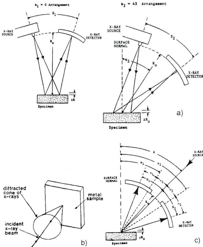
Fig 10 Schematic diagrams of X-ray technique arrangements a) double-exposure arrangement; b) cone of diffracted beams produced by a single X-ray beam; c) single-exposure arrangement,  $R_0$  the specimen - to - detector radius
