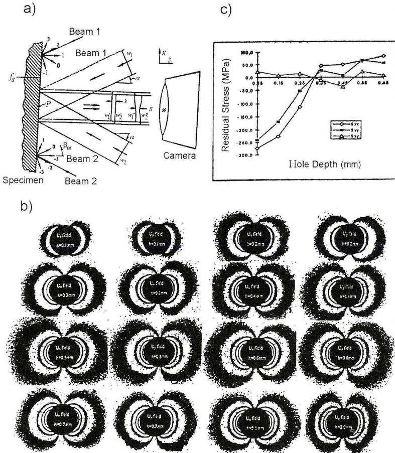
Fig. 6 The hole drilling method: surface displacement measurements provided by moiré interferometry (according to Ref. [15]); a) the principle of the measurement, b) displacements contour maps, c) the residual stress distribution inside the material
