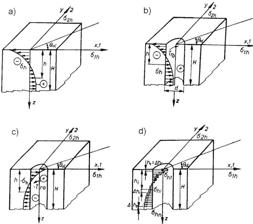
Fig. 4 The principle of the hole-drilling method (according to Ref. [9]); a) residual stress existing in the material, b) the reactions which should be applied at the surface of the drilled hole, c) applying the stresses with opposite sign, d) approximation of the real stress distribution
