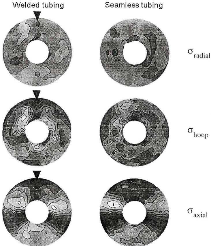
Fig. 12 Neutron diffraction residual stress measurement results for a bent welded tube and a bent seamless tube; white = - 400 MPa, black = 400 MPa (according Ref. [34])
