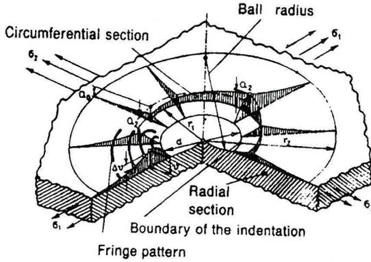
Fig. 7 The nondestructive penetration method (according to Ref. [23]): a typical picture of plastic deformation around an indentation
