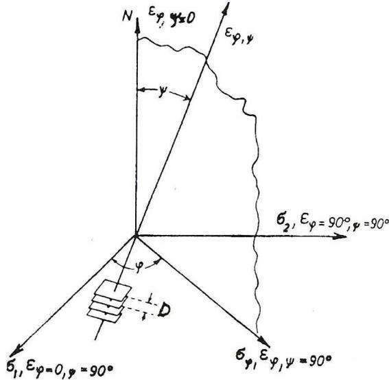
Fig. 9 Symbols used in X-ray strain measurement
