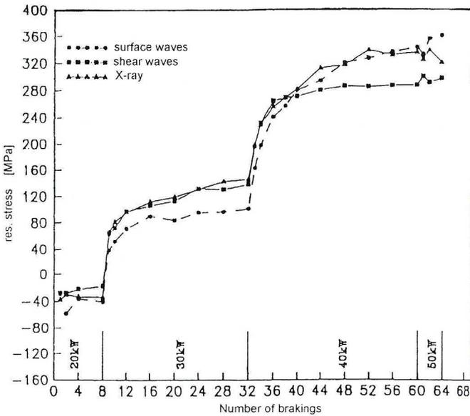
Fig. 14 The change in the circumferential residual stress component in the train wheel head due to multiple brakings of different power
