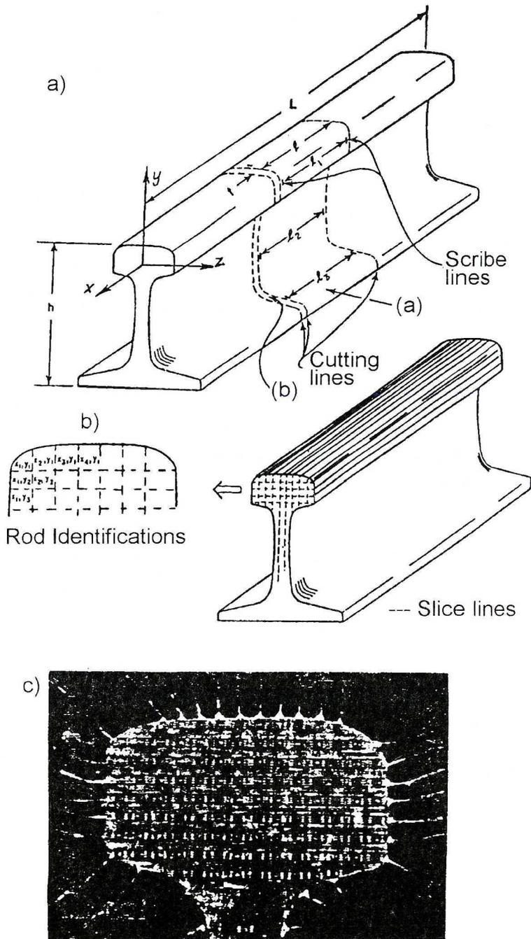
Fig. 1 The sectioning method for determining residual stress in rails (according to Ref. [2]), a) two specimen cut out from a rail portion, b) sectioning of the specimen (a) into long bars, c) rosettes of strain gages at the face of the thin slice
