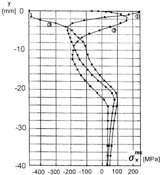
Fig. 15 The 2-D residual stress distribution due to the friction elastic-plastic rolling process of the steel strip, obtained by the FEM computation (according to Ref. [41]): ① - free rolling, ② - rolling with braking (75%), ③ - rolling with acceleration (75%)
