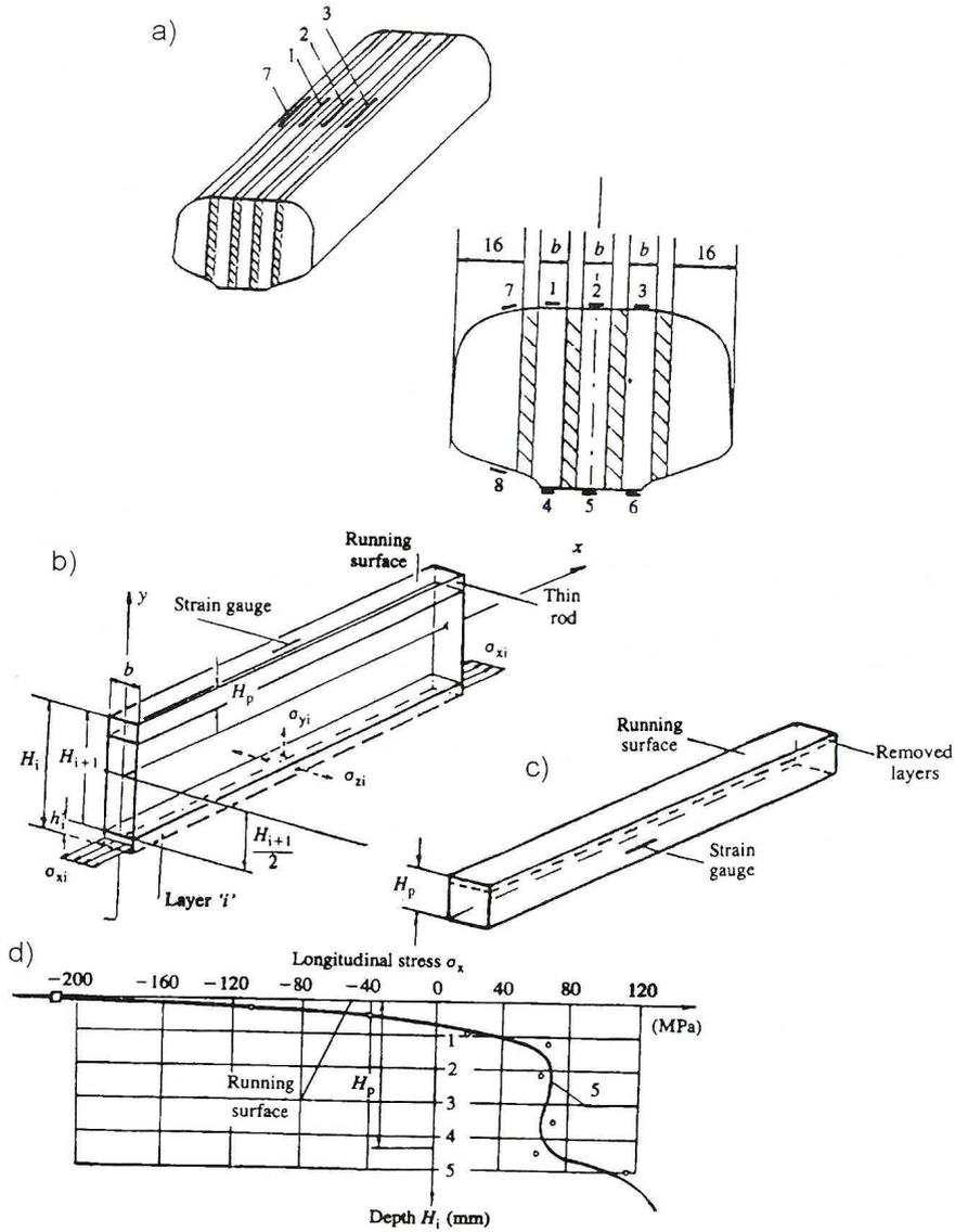
Fig. 3 The sectioning / layer removing method for determining residual stress in a rail head (according to ref. [4]): a) cutting the rail head into plates; positions of strain gages, b) process of plate sectioning: removing layers, c) process of removing layers from the thin bar, d) distribution of longitudinal ( $\sigma_x$ ) stresses along the centreline if the rail head cross section in the vicinity of the running surface
