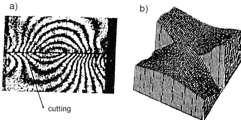
Fig. 17 The hybrid method for determining residual stress in the laser weld (according to Ref. [45]); a) the contour map of the displacement obtained by the moiré interferometry, b) the spacial shape of the displacement field
