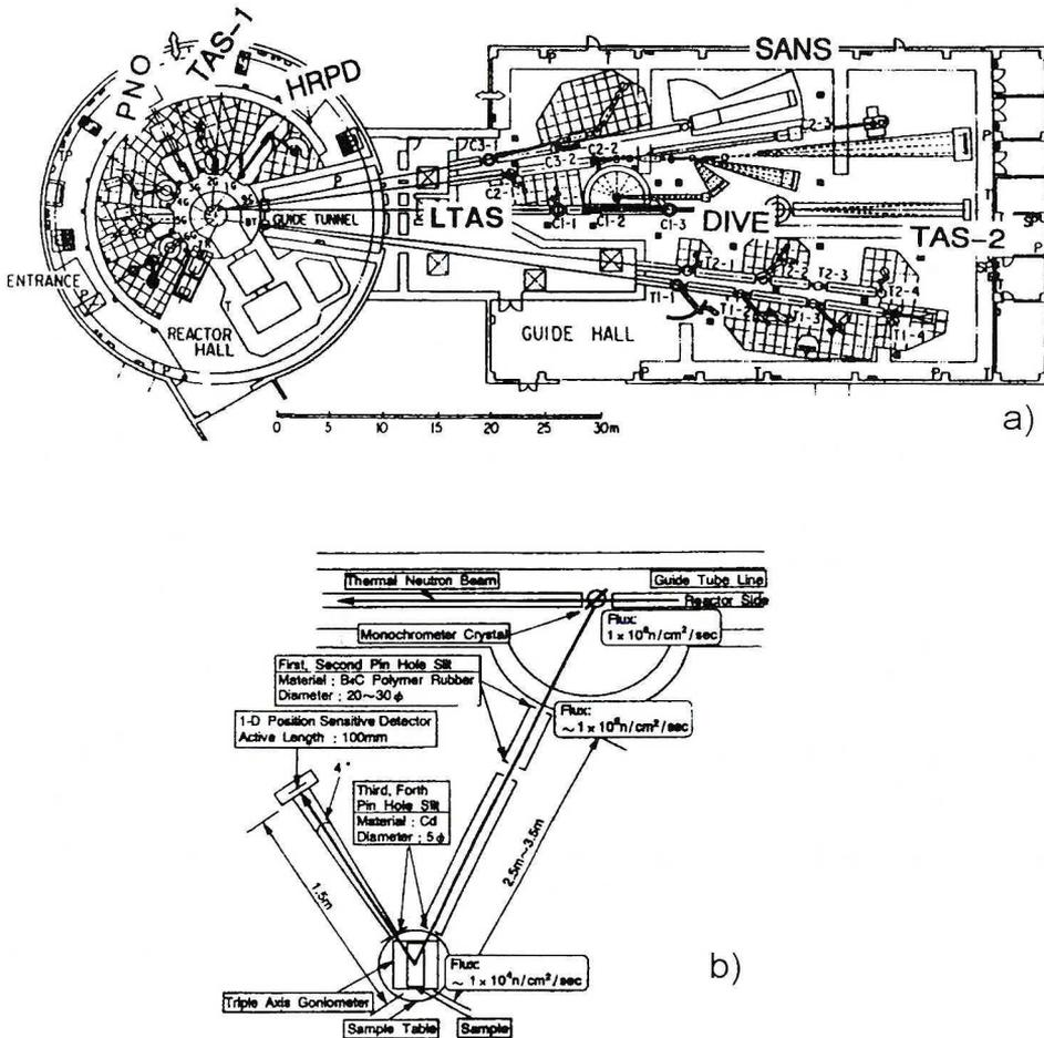
Fig. 11 Neutron diffraction arrangements in Tokai Establishment of Japan Atomic Energy Research Institute (according to Ref. [30]); a) outline of Japan Research Reactor - 3M; b) outline of neutron diffraction apparatus
