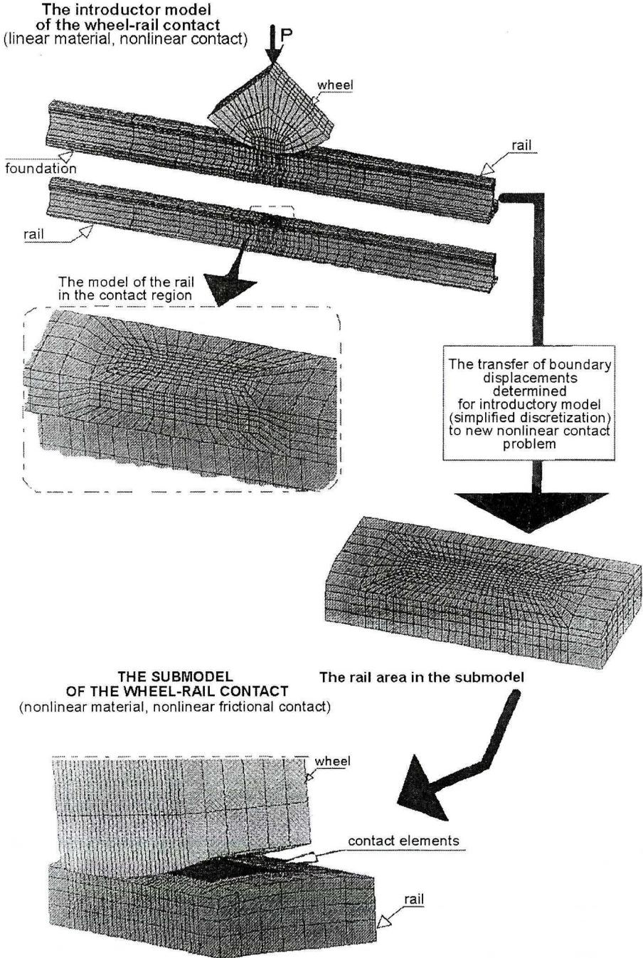
Fig. 16 The way of searching for the 3D numerical solution of the elastic-plastic rolling contact problem: (according to Ref. [42])
