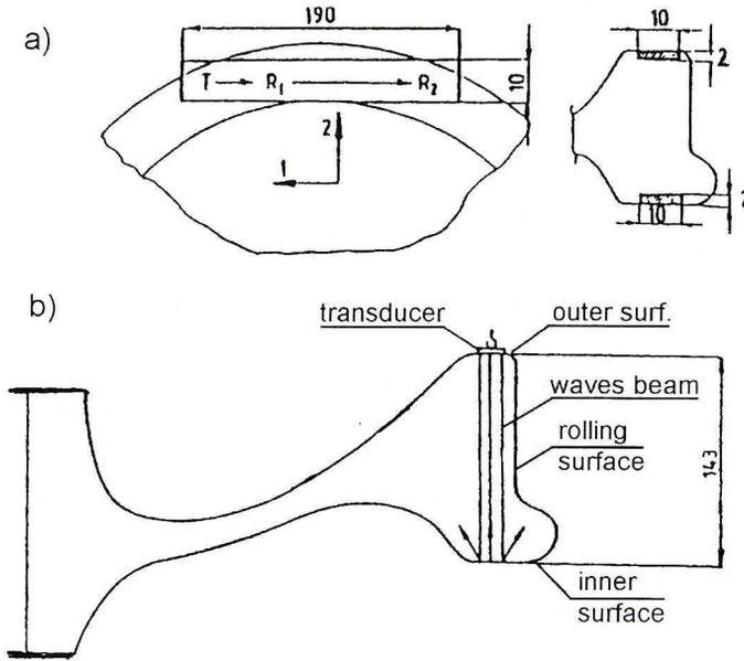
Fig. 13 Ultrasonic techniques for residual stress measurements in train wheels a) surface waves arrangement; b) bulk shear waves arrangement
