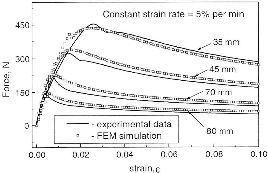
Fig. 7 FE prediction of buckling behaviour of HDPE strips of different length
