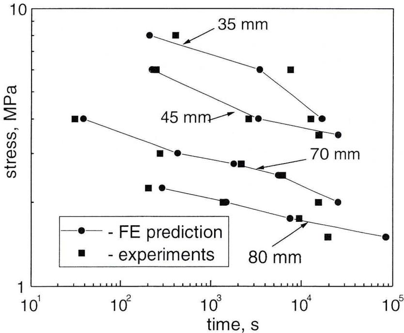
Fig. 10 FE prediction vs. experimental data on the periods till buckling onset in HDPE strips of different lengths under constant compressive loading
