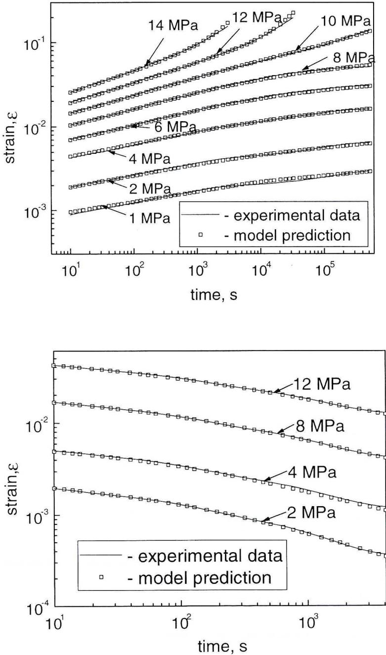
Fig. 1 Experimental data [6] and model prediction for the creep and recovery behaviour of HDPE
