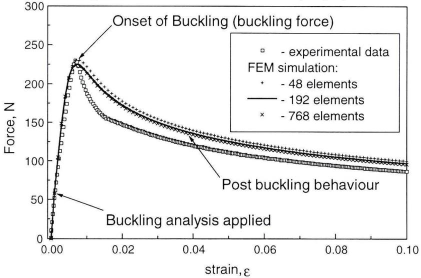
Fig. 5 Simulation of buckling and post buckling behaviour of 70 mm long strip (strain rate of 5% per minute), using mesh with different number of elements
