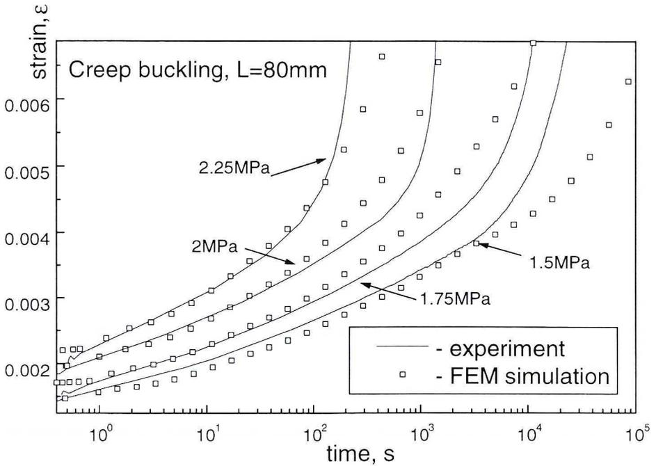
Fig. 9 Experimental data and FE prediction for the compressive creep of HDPE strips
