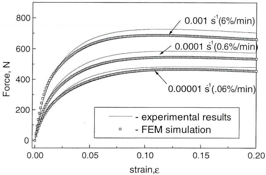
Fig. 2 FE simulation of ramp tensile tests on HDPE
