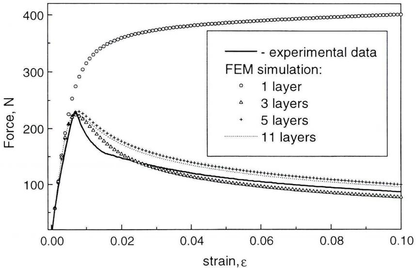
Fig. 6 Simulation of buckling and post buckling behaviour of HDPE strip, using shell elements with different number of layers
