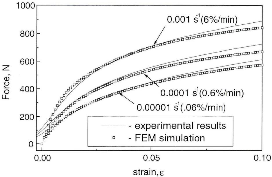
Fig. 3 FE simulation and experimental results of ramp compression tests of HDPE for three different strain rates
