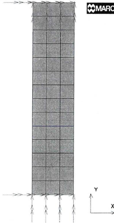
Fig. 4 The scheme of mesh and boundary conditions of the 70 mm long specimen
