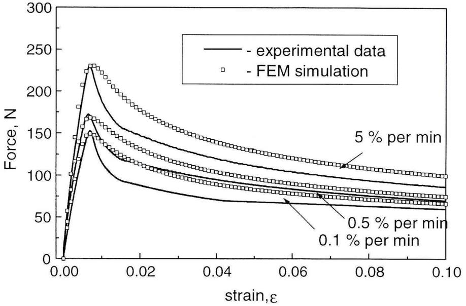
Fig. 8 Prediction of buckling force for the HDPE strip loaded by three different strain rates
