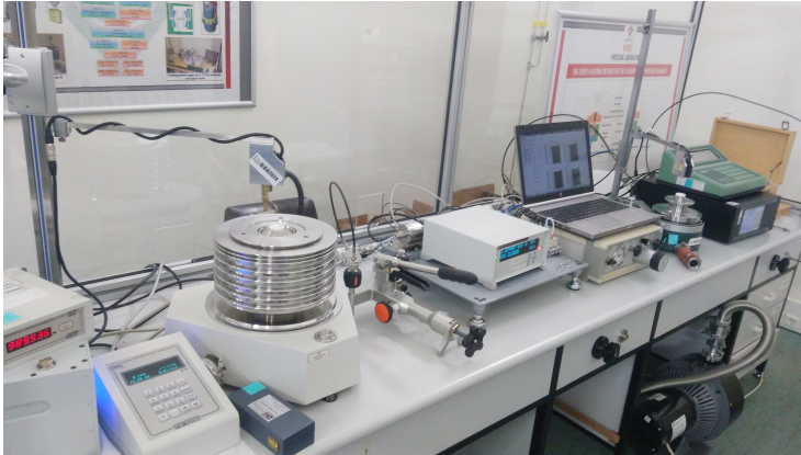
Fig. 3. Cross-floating and digital manometer-assisted calibration setup.
