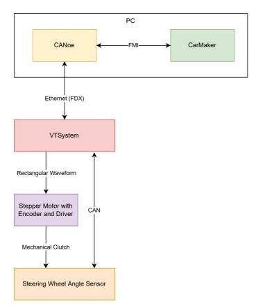
Fig. 3. Testbench diagram including the communication protocols used.
