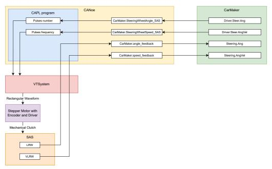
Fig. 7. Flow and mapping of variables between the test system components.
