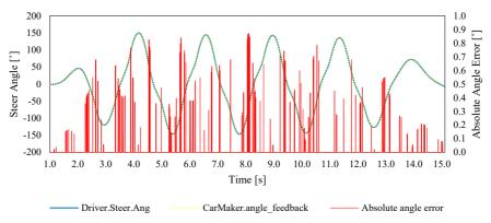
Fig. 9. Superimposed CarMaker transmitted and received angle waveforms and absolute angle error.
