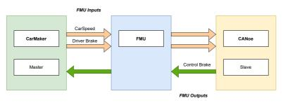
Fig. 5. Scheme of communication between CarMaker and CANoe using FMU in the master-slave architecture.
