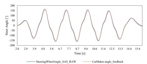
Fig. 14. The steering wheel angle requested by the driver and the angle measured by SAS III.
