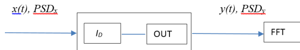
Fig. 4. Setup to evaluate the noises at the detector whose output circuit is connected to a FFT analyser.
