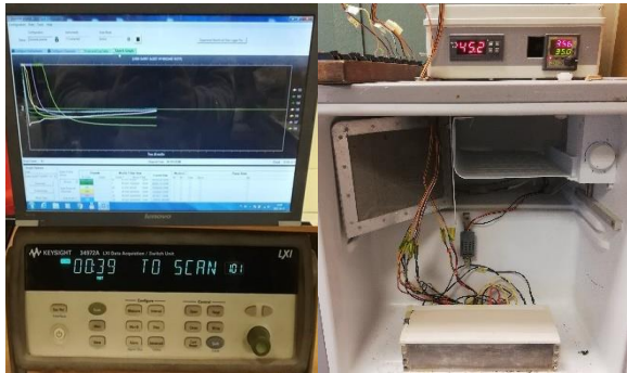
Fig. 5. Keysight recorder with computerized data logging (left), climate chamber (right)
