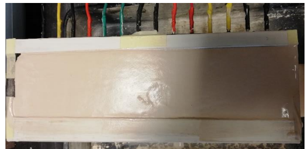
Fig. 4. Core with protective coating applied by pouring
