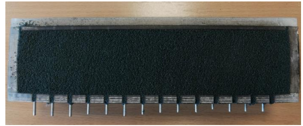
Fig. 2. Test core with formed electrodes
