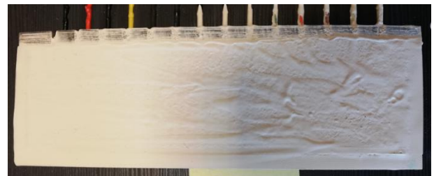
Fig. 3. Core with protective coating applied by dipping
