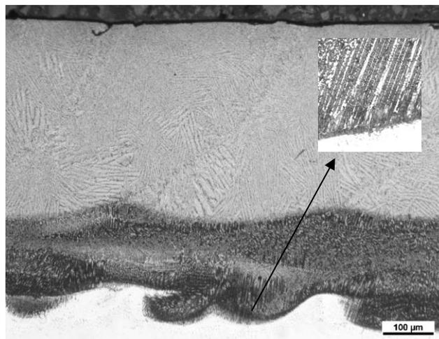
Fig. 1. Microstructure of NiCrAlY coating is as-clad state on 316L alloy
