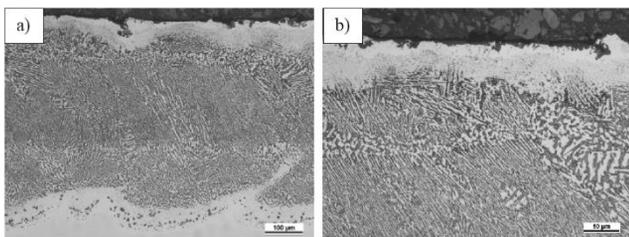
Fig. 7. Microstructure of NiCrAlY coating on 316L alloy after annealing at 1000°C/100h
