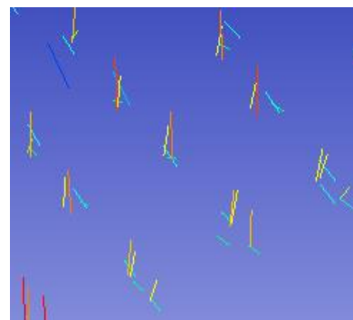
Fig. 7. Deviations represented in the FI software by lines: points next to each other characterized by positive (warm colours) and negative (cool colours) deviations
