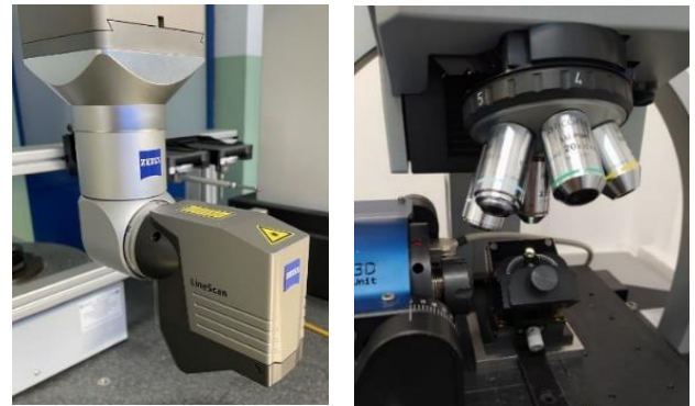
Fig. 2. The LineScan probe (left) and measurements of the insert conducted by using the InfiniteFocus microscope (right)
