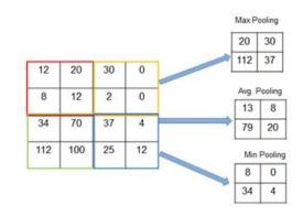
Fig. 6. Types of Pooling
