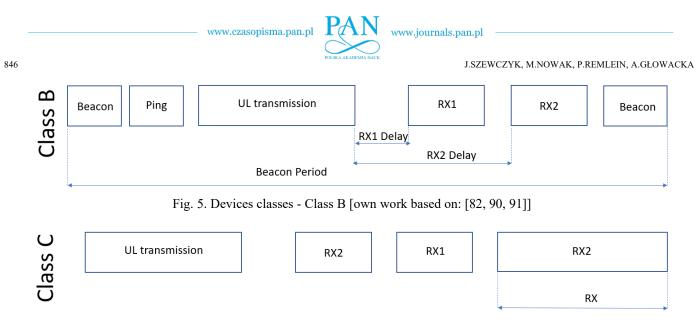
Fig. 6. Devices classes - Class C [own work based on: [82, 90, 91]]
