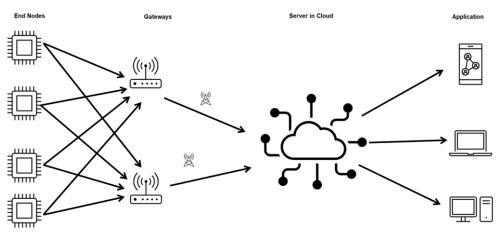
Fig. 2. LoRaWAN architecture [own work]
