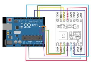
Fig. 9. Schematic of the Arduino's connection to the RFM95W. Source: own elaboration based on: [89]
