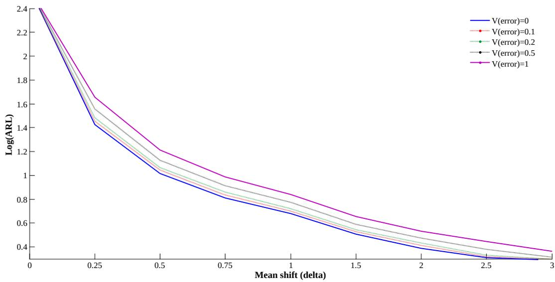
Fig. 1. The ARL values corresponding mean shifts
