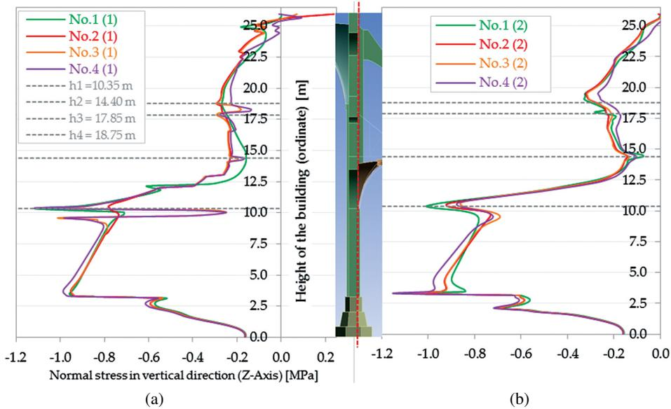
Fig. 10. Normal stresses in the vertical direction along the height of the wall and pillar along the lines running along the external face of the wall structure: a) in the axis of the cross-section through the pilaster; b) on the edge of the pillar
