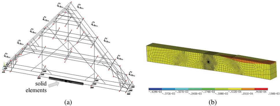
Fig. 1. An example of modelling a connection using beam and solid elements [24]:
