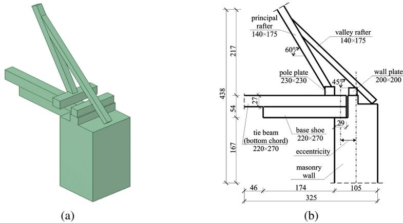
Fig. 6. Supporting a roof truss on masonry walls: a) three-dimensional geometric model of a separated structure strip, b) 2D sketch with marked structural elements of the connection
