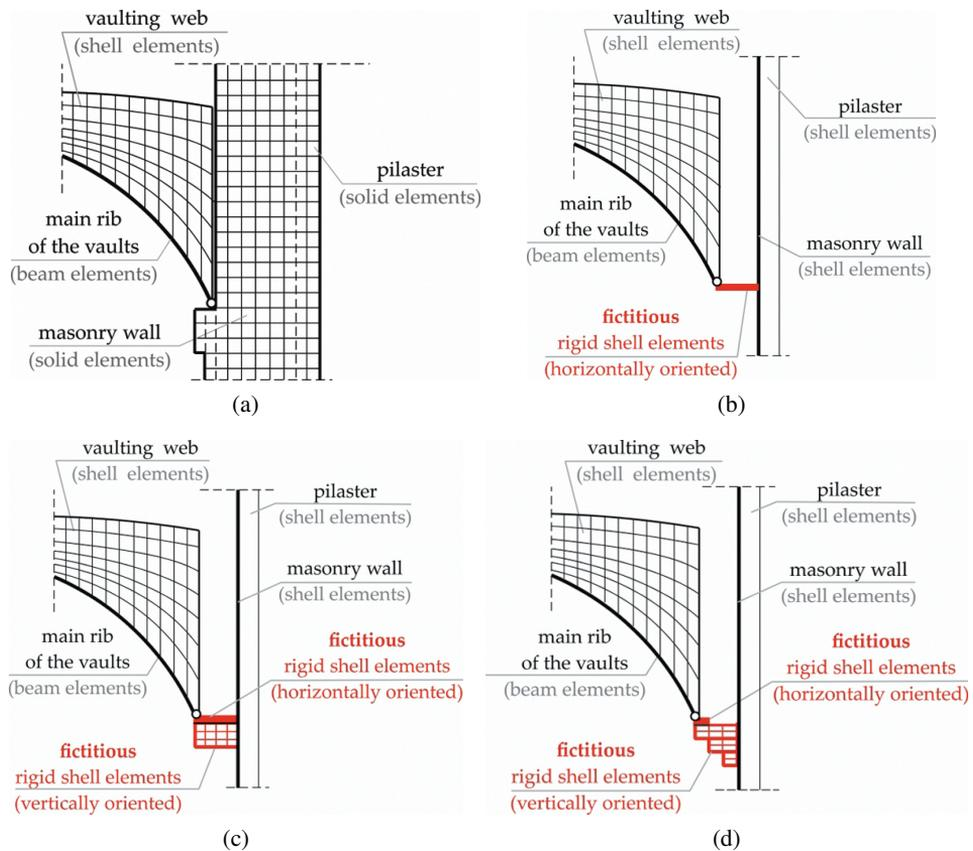
Fig. 8. Static schemes of the connection of the main ribs and vaults with the walls and the rigid fictitious elements used in the models: a) reference model No. 1, b) model No. 2, c) model No. 3, d) model No. 4
