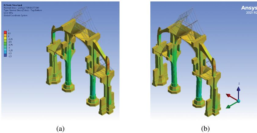
Fig. 9. The stress-deformation behavior of the structure: a) reference model – No. 1 (walls modelled with solid elements), b) model No. 4
