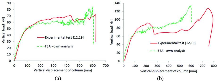
Fig. 6. Response curve load-vertical displacement of specimen with: a) flush end-plate, b) extended end-plate
