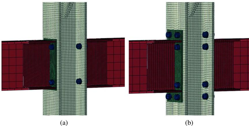
Fig. 5. Detailed view of: a) flush, b) extended end-plate joint with mesh
