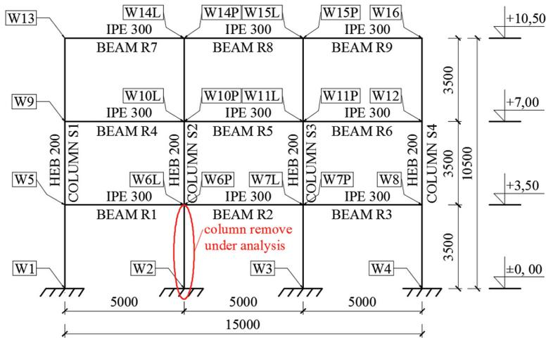
Fig. 9. Static diagram of the analyzed frame
