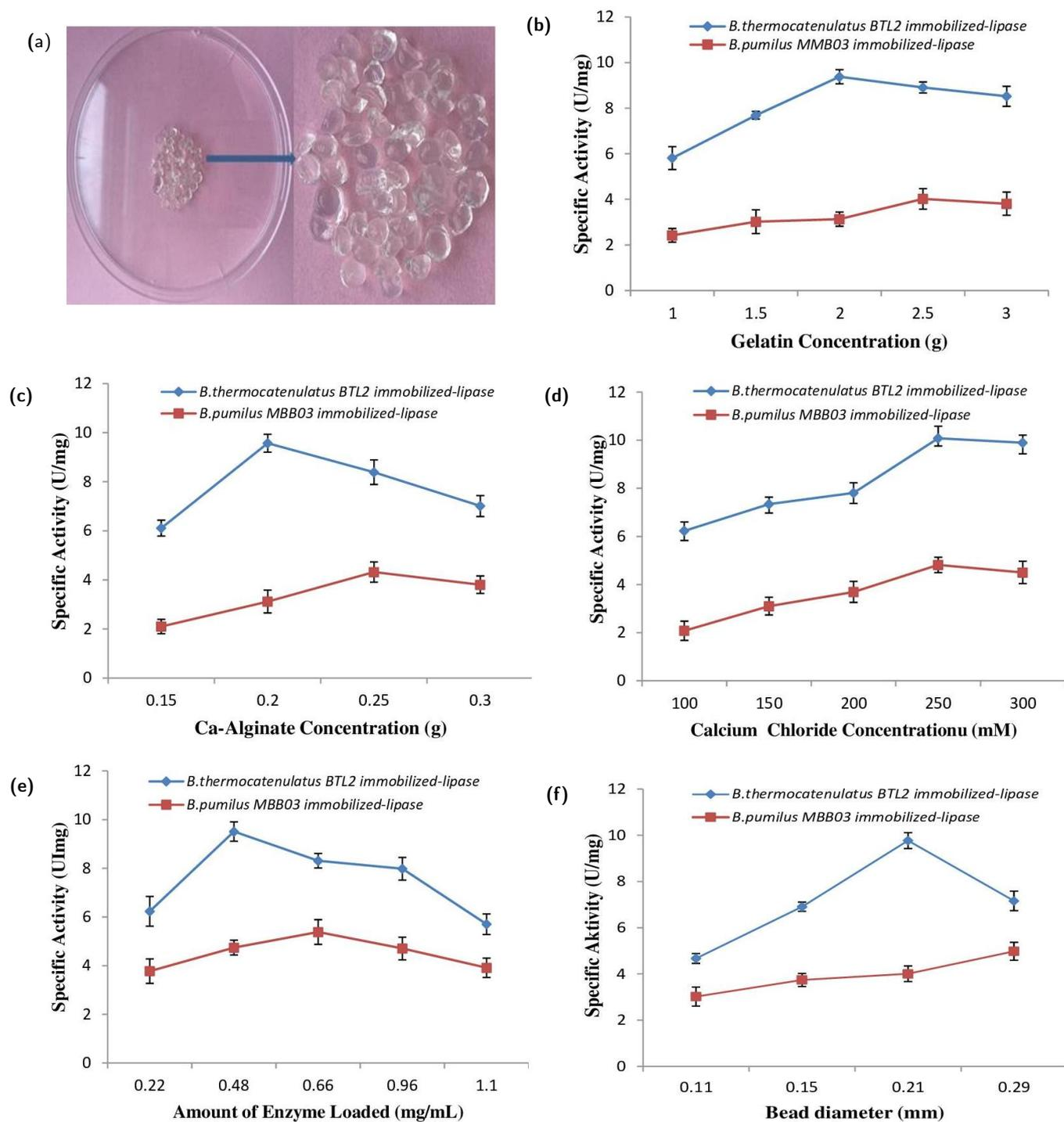
Figure 1. Hydrogel beads obtained by of *B. thermocatenulatus* BTL2 and *B. pumilus* MBB03 immobilized-lipases in Ca-Alg@gelatin mixtures (a). The effect of gelatin concentration (b), alginate concentration (c), CaCl<sub>2</sub> concentration (d), enzyme concentration (e) and bead size (f) on the immobilization of *B. thermocatenulatus* BTL2 and *B. pumilus* MBB03 lipases in Ca-Alg@gelatin mixtures.
