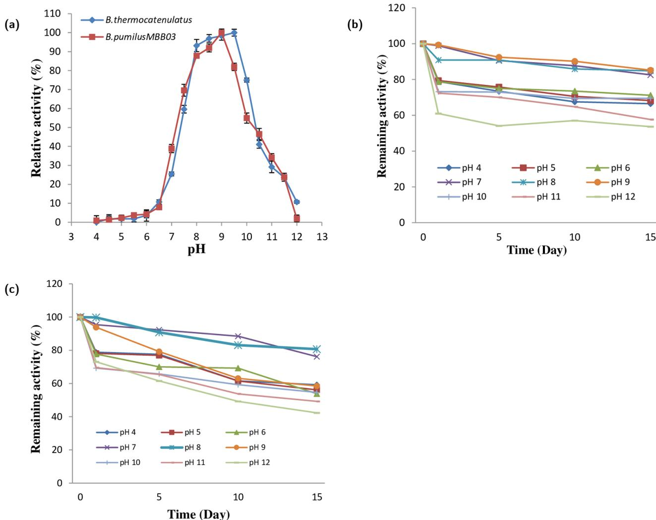
Figure 2. Effects of pH on *B. thermocatenulatus* BTL2 and *B. pumilus* MBB03 immobilized-lipase activities (a). Effects of pH on *B. thermocatenulatus* BTL2 immobilized-lipase (b) and *B. pumilus* MBB03 immobilized-lipase stability (c). pH 9.5 for *B. thermocatenulatus* BTL2 and pH 8.5 for *B. pumilus* MBB03 immobilized-lipase was taken as 100%.
