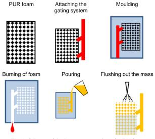
Fig. 1. Scheme of the investment casting of AZ91foam
