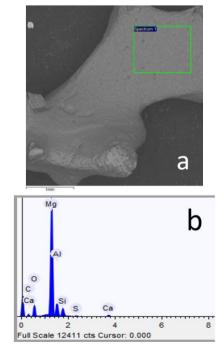
Fig. 5. Chemical analysis of the strut surface confirming elements originated from the moulding materials
