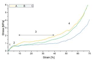
Fig. 7. Stress-strain curves of AZ91 foam samples, performing with typical for metallic foams regions: 1 – elastic strain, 2 – plastic bulking, 3 – plateau phase, 4 – densification
