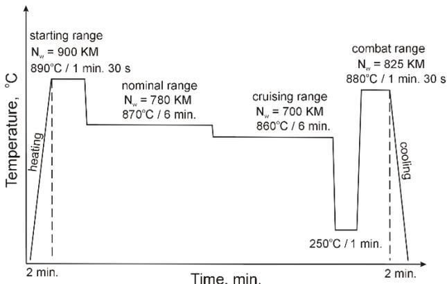
Fig. 1. Diagram of the basic high temperature cycle of the equivalent durability test of an aircraft engine PZL-10W and the values of power at the main engine shaft corresponding to its individual stages,  $N_w$  and the values of the internal temperature of the engine combustion chamber glow tube
