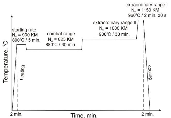
Fig 3. Diagram of the high temperature cycle with a pronounced extraordinary range II and extraordinary range I of the equivalent durability test of an aircraft engine PZL-10W and the values of power at the main engine shaft corresponding to its individual stages,  $N_w$  and the values of the internal temperature of the engine combustion chamber glow tube
