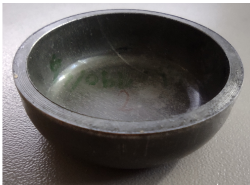
Fig. 15. The appearance of the exemplary (6082 T4) cup edge after drawing
