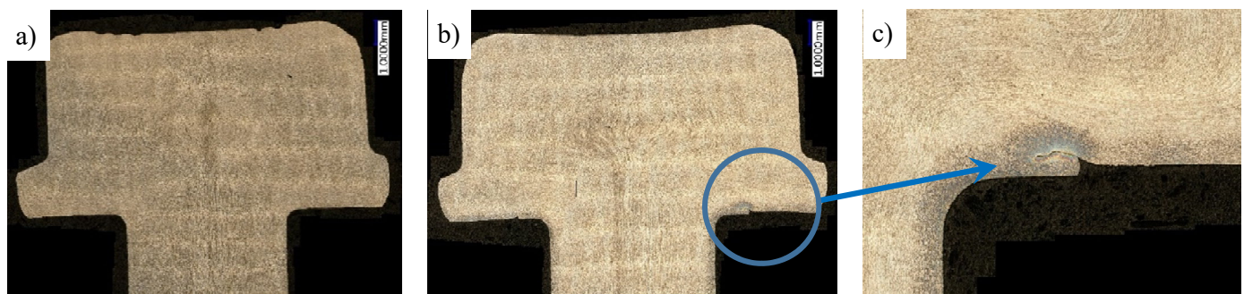
Fig. 1. Samples of polished longitudinal sections of DIN 6921 M6x20 bolts after the forging process with the grain flow pattern. a) variant compatible with the technology used, b) variant with a deliberate defect of lap forging the bearing surface, c) the lap forging of the bearing surface
