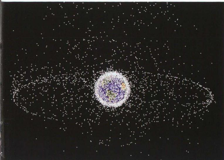
Numerous satellites and high volumes of space debris are present in geosynchronous orbits, particularly orbits at approx. 35,785 km above Earth's surface (computer simulation)
