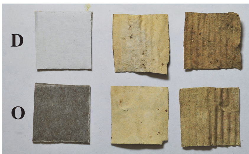
Fig. 1. PB samples before (B) and after (A) the 1-month experiment in sandy soil
