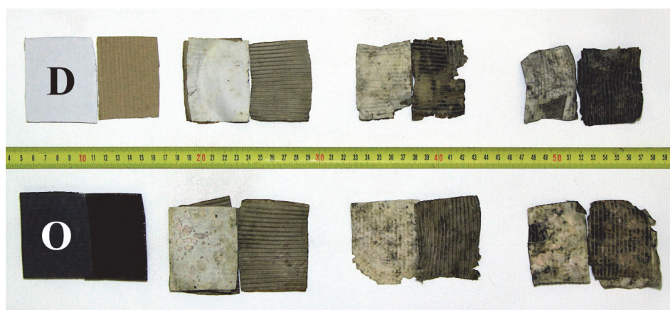
Fig. 3. Dry (D) and oiled (O) PB samples after 0, 2, 4, and 6 weeks in leaf mold
