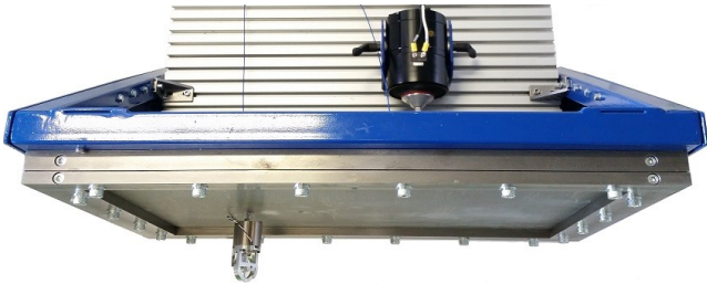
Fig. 4. Picture of the test setup used to assess the control performance of the closed loop sensor-actuator for the voltage-driven proof mass actuators
