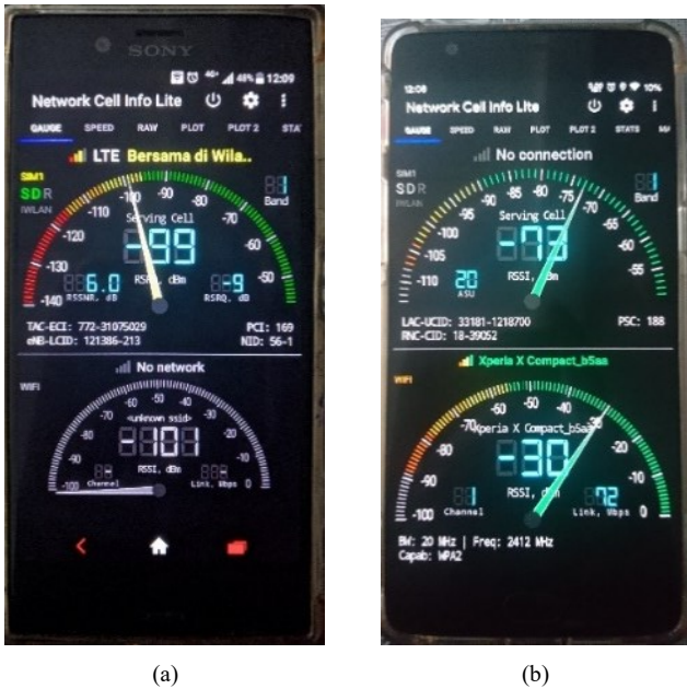
Fig. 3. (a) Smartphone as an access point (b) Smartphone as receiver
