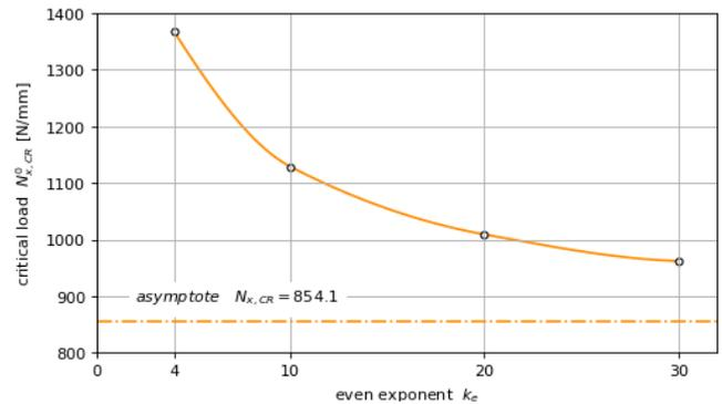
**Fig. 9.** The graph of the critical load of the exemplary square sandwich plate ( $e_0 = 1/20$ )
