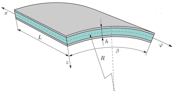
Fig. 1. Scheme of the sandwich cylindrical panel
